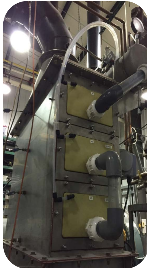
Figure 7-3. Lab TMC unit as installed with new TMC modules (left before water connections, right after water connections)
