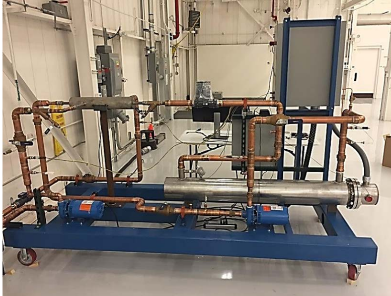
Figure 5. A picture of the completed water-water heat exchanger test loop at Sandia's NESL.
