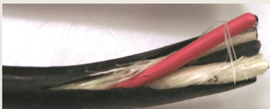
Brand-Rex Cable 300 kGy, 340 Gy/hr (2/20/15) Accelerated testing
