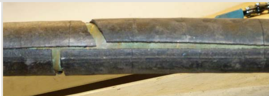
Actual cable failure (aged neoprene jacket)
