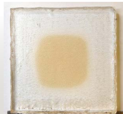
Picture of Xe Arc Aged Coupon: Glass-EVA-Glass, ~65 x 65 mm
