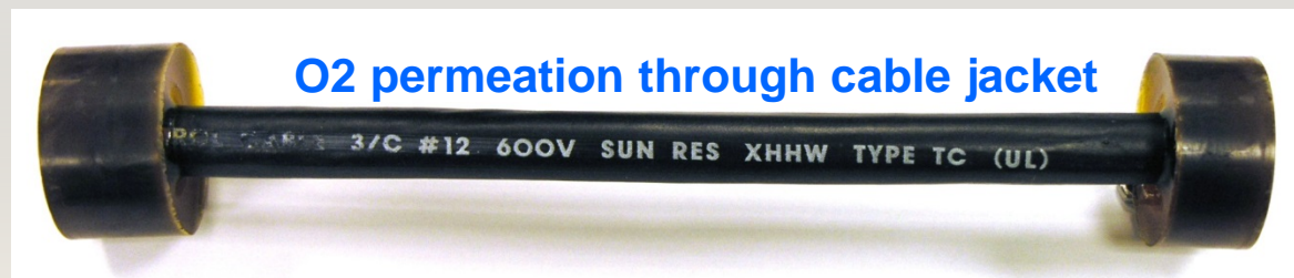
Brand-Rex Cable 300 kGy, 340 Gy/hr (2/20/15) Accelerated testing
