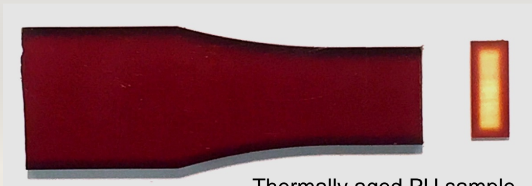
Thermally aged PU sample from aging tests supporting material selection/qualification
