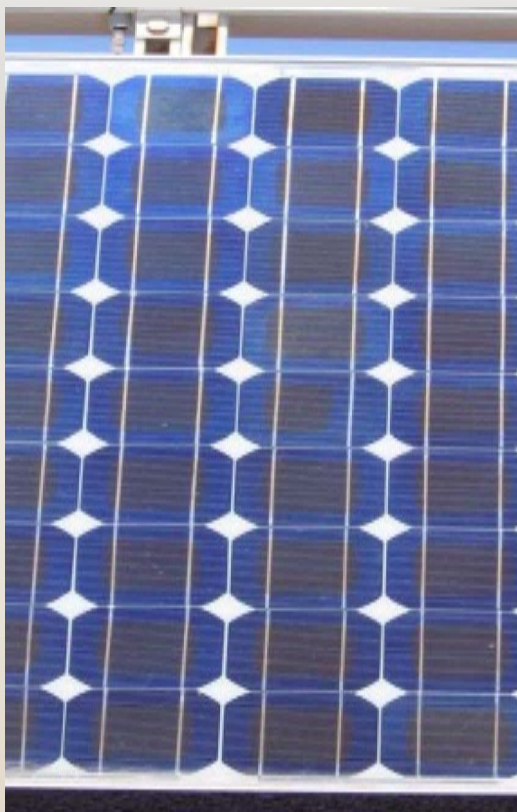
PV Module, ~15 years Arizona. Encapsulant is PHOTOCAP 15295
