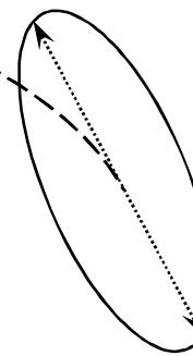
Two (opposite) velocity error directions which result in no displacement of the trajectory (except in time)
