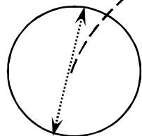
Body orientation remains inertially stable outside the atmosphere
