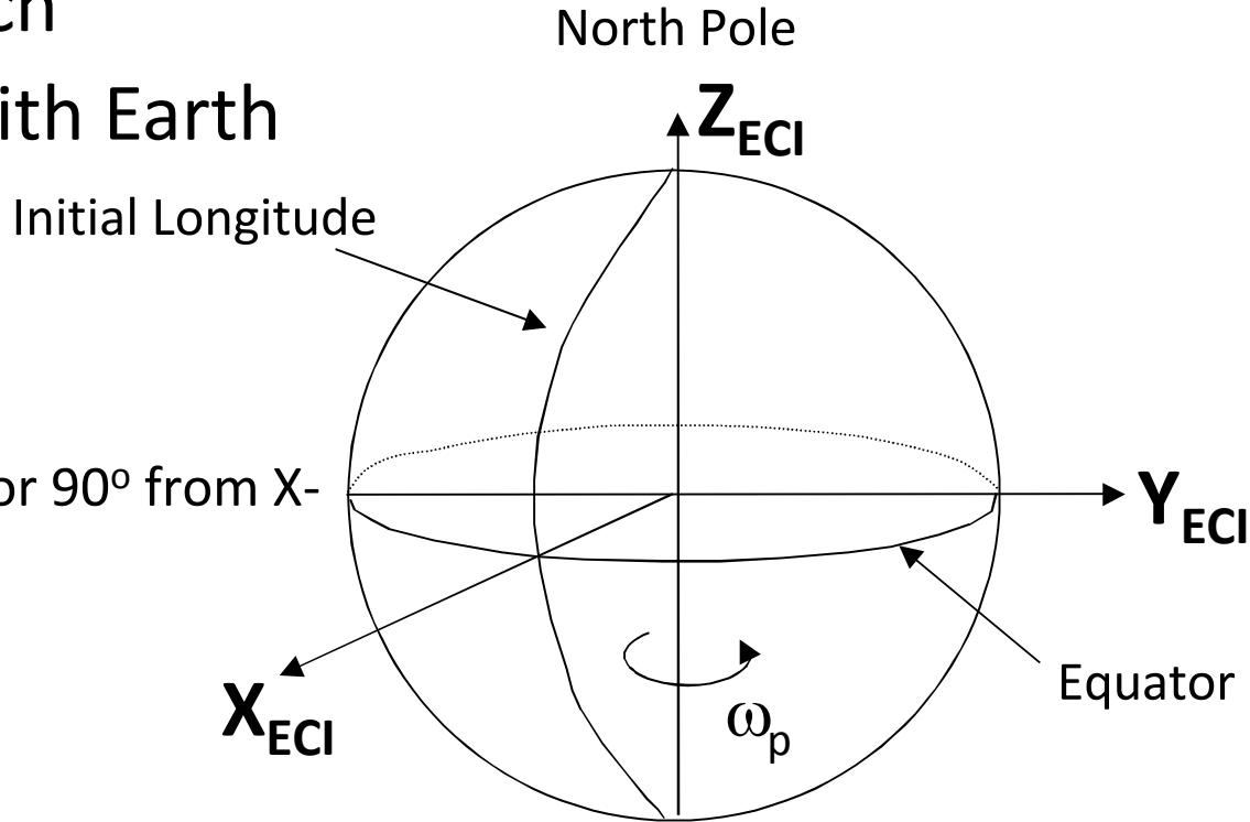
Other Names: Inertial (I), Earth-Centered Inertial
