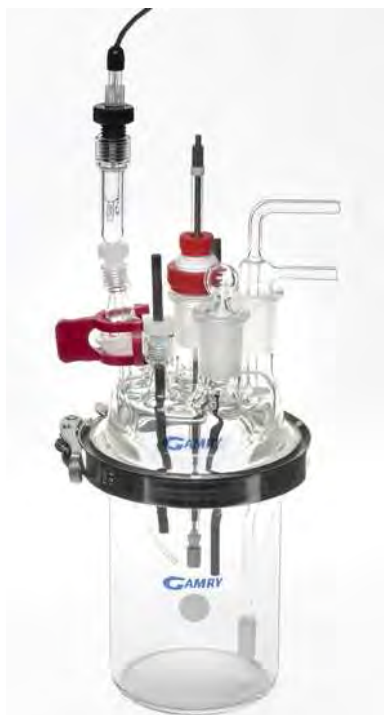
Figure S3.13: Gamry 1 L Multiport Corrosion Cell with Interface 1000 potentiostat control (not shown).
