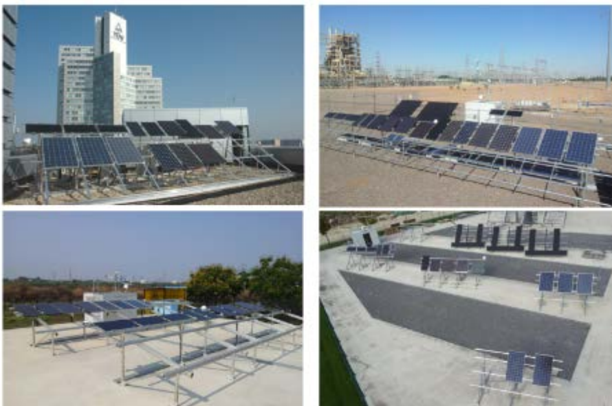
Figure 35: Outdoor test installations in Germany, Arizona, India and Italy with 15 PV modules operating since 2014.
