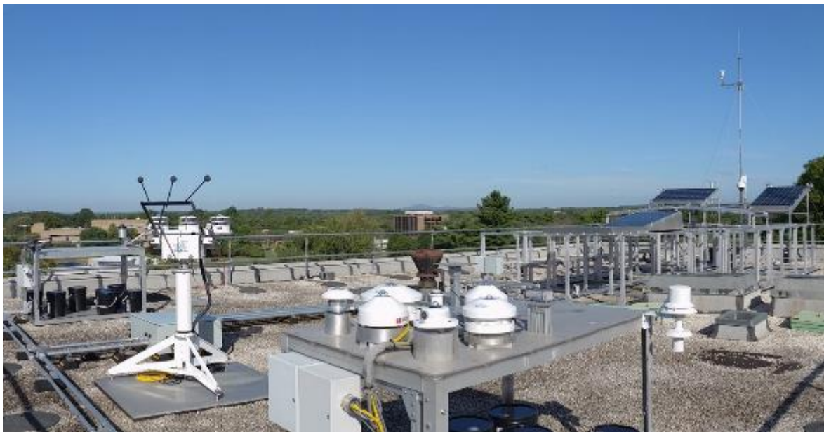
Figure 62: The weather station, showing the various stationary and sun-tracking instruments as well as the I-V traced reference modules.
