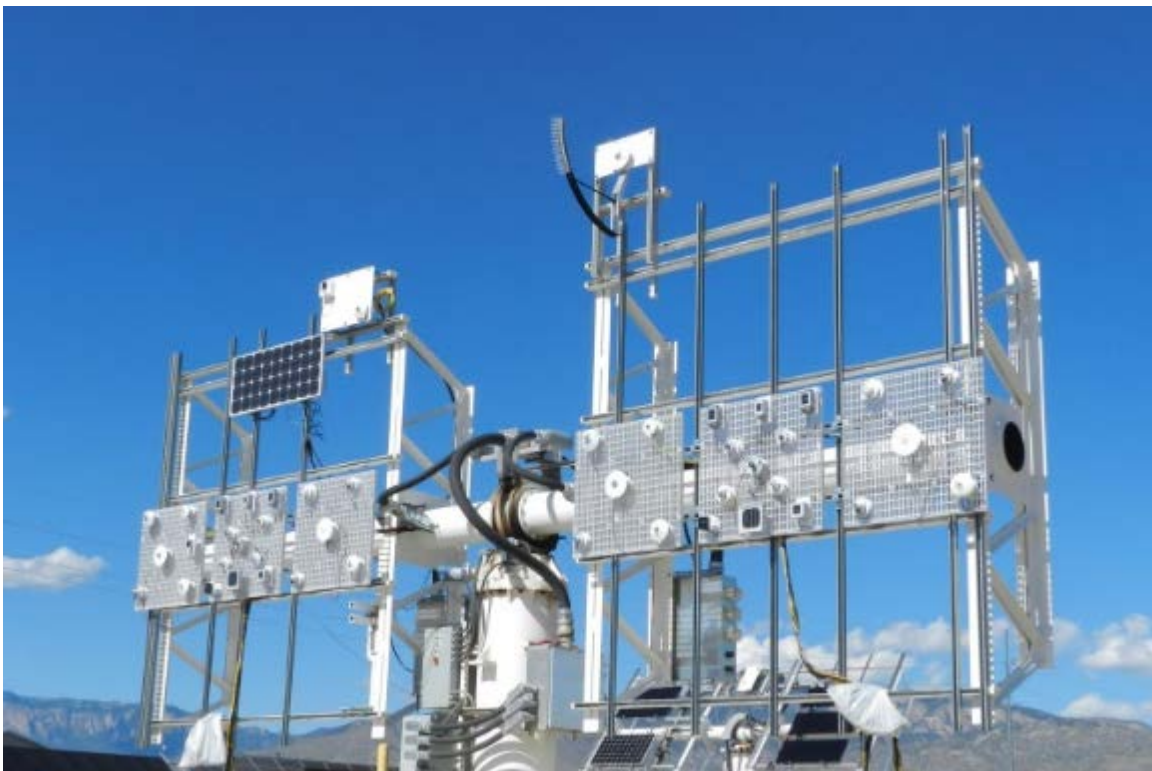
Figure 22: Two sets of sensors mounted on a two-axis tracker at Sandia National Laboratories.
