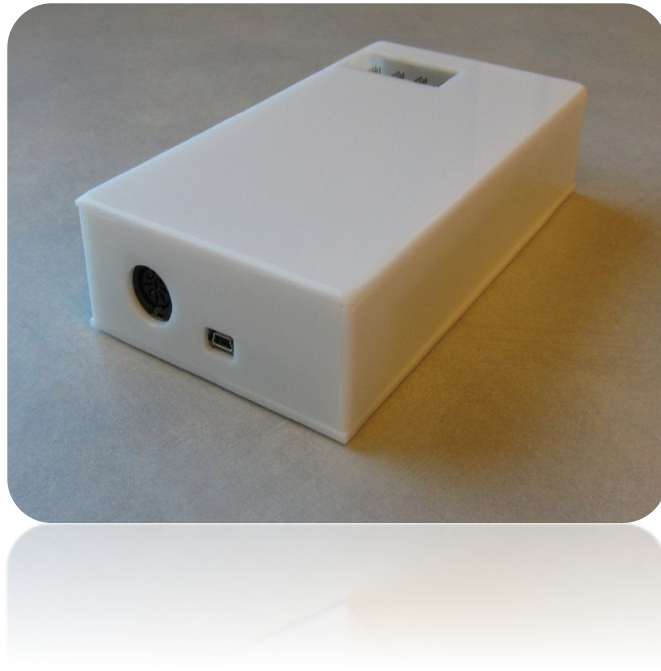
Figure 10. A new versatile stimulation system box built using the stimulation IC with full software features support running on Windows workstation.
