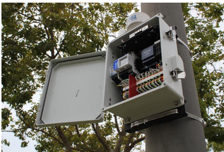
Figure 2: A \mu PMU installed on a utility electric distribution pole. The device consists of a high-resolution power quality monitor and a GPS antenna (mounted on top of the box in this installation).
