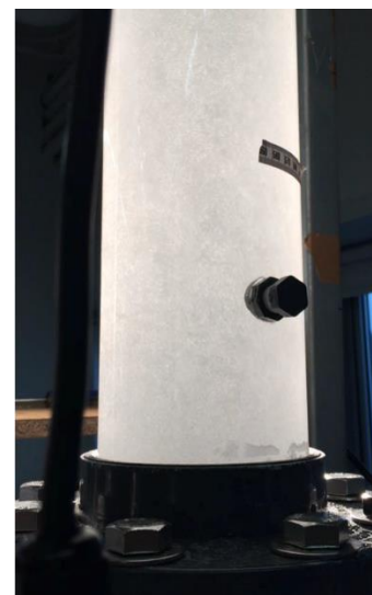
Figure 1: Picture of test reactor showing very fine bubble distribution.
