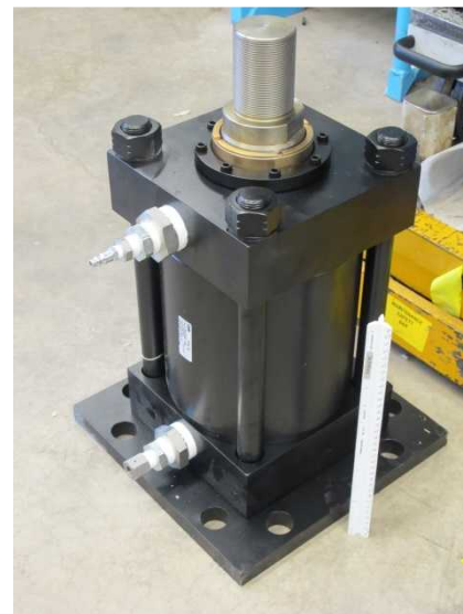
Fig. 9. High volume hydraulic piston used to generate hydrostatic pressure for \frac{1}{4} -scale tests. The piston was selected to eliminate restroking during pressurization.
