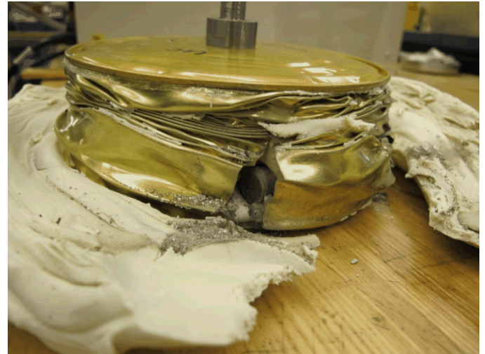
Fig. 15. Typical post-test 1/4-scale sample showing split along side of sample. White material around sample is clay used to seal the breaches in sample during testing. Full-scale uniaxial samples did not typically split but rather developed pinholes leaks.
