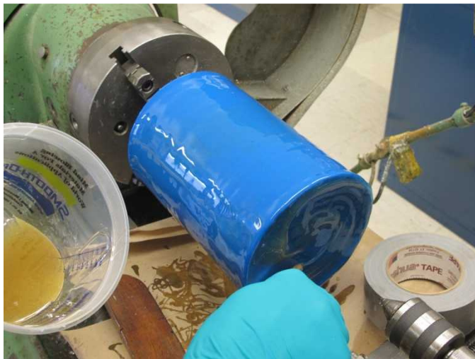
Fig. 5. Hydrostatic sample (1/4-scale) being coated with PMC®-770 urethane rubber over the three coats of Color Guard and two layers of Kevlar® sheets.
