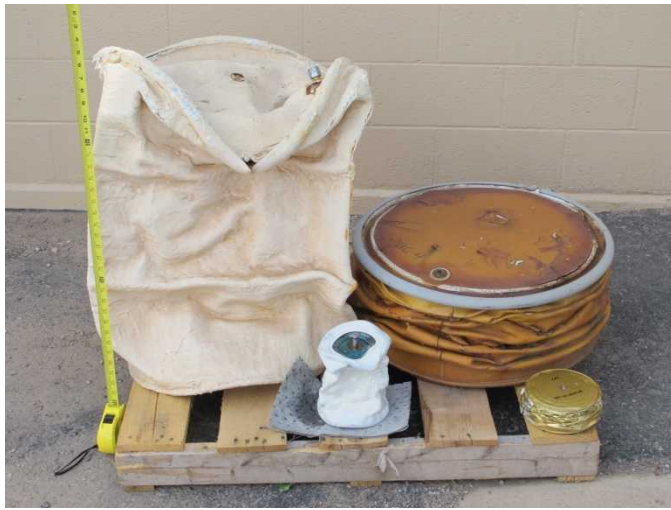
Fig. 17. Comparison of full-scale and \frac{1}{4} -scale hydrostatic (left) and uniaxial samples (right). Note different jacket material used for each test configuration.
