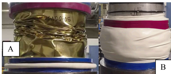
Fig. 2. A) \frac{1}{4} -scale uniaxial test before jacketing and B) after clay and balloon jacketing.
