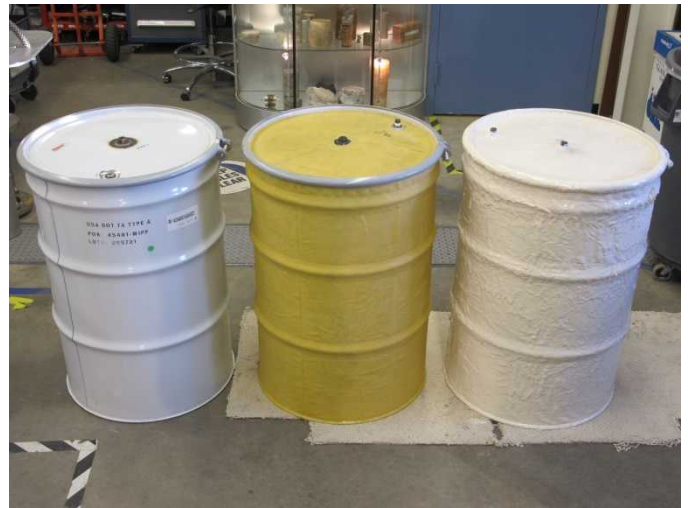
Fig. 6. Full scale Hydrostatic sample with no jacket on left, wrapped with Kevlar® and one coat of PMC®-770 center and multiple coats of Brush-On®40 right.
