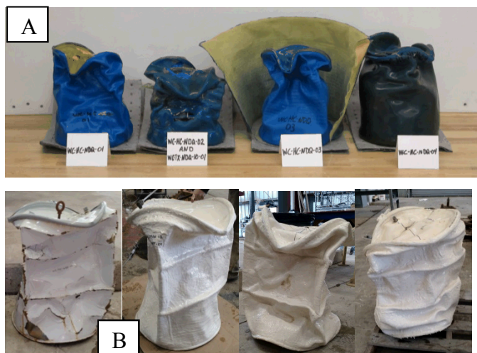
Fig. 22. Posttest \frac{1}{4} -scale (A) and full-scale (B) hydrostatic compression samples. Samples in numerical order from left to right.
