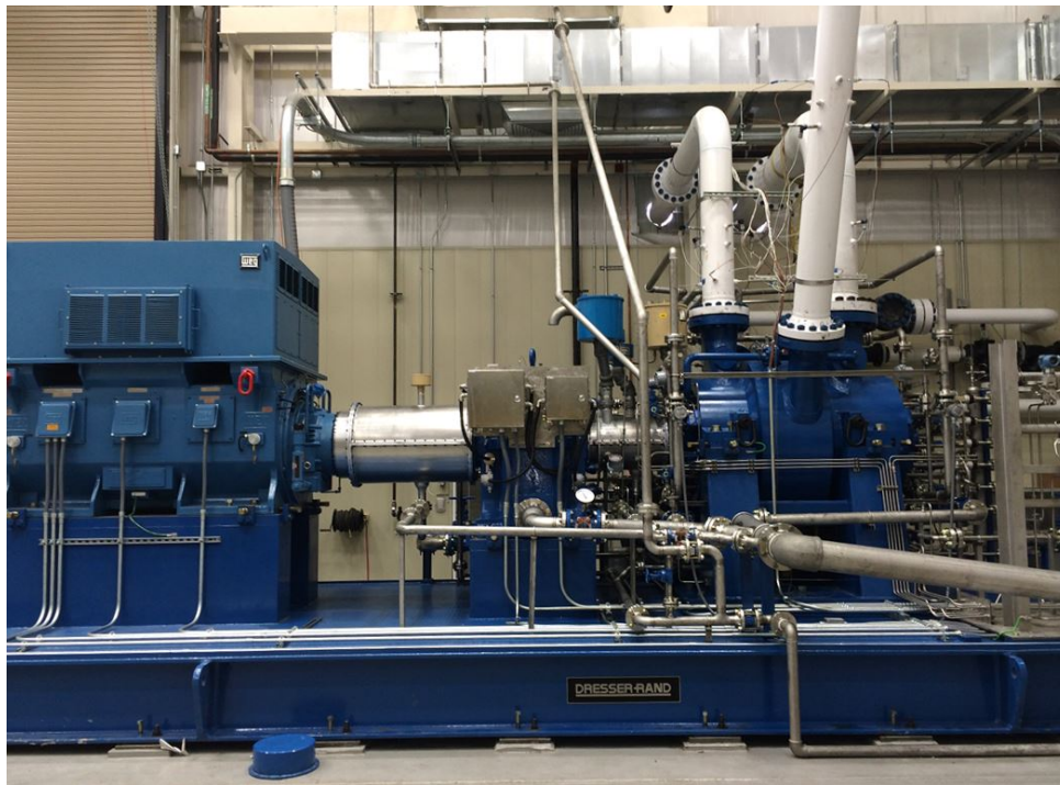
Figure 2-98. 3-MW CO 2 Compressor Located at SwRI Turbomachinery Research Laboratory
