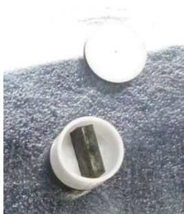
Figure 2. Sample Measuring 3 mm x 5 mm x 1 mm Inside the Crucible
