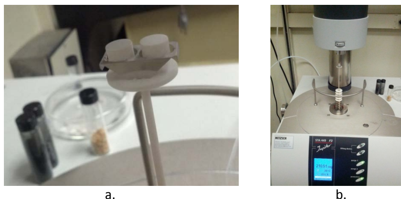
Figure 4. a. and b. Sample Crucibles Mounted in Netzsch TGA Machine
