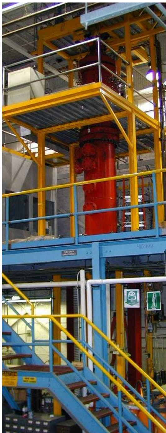
Figure 1. The Pressurized Entrained Flow Reactor at Georgia Institute of Technology. Diagram of the pressurized entrained-flow reactor (PEFR). The height of the reactor section is 2 m whereas the height of the whole equipment including the biomass feed system and the collector and gas sampling assembly (not shown in the schematic drawing) is 12 m.
