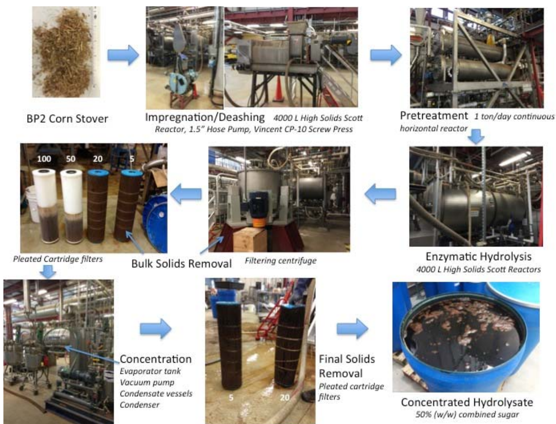
Figure B.3.1.1. Deconstruction process flow pictures of concentrated hydrolysate production for the Final validation and January 2015 production run. Numbers above or below the pleated cartridge filters represent the filter pore size in microns. The concentrated hydrolysate production process for the May and October 2014 campaigns differ in the bulk solids removal step, which was only conducted in the filtering centrifuge for these runs.
