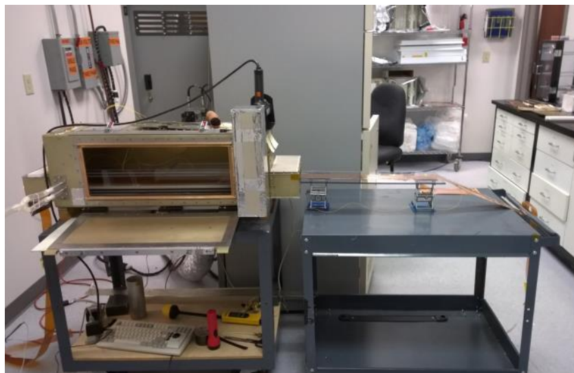
Figure 2: The digital image shows the tall MC2100 delivering VFM power in the chamber with chokes on both ends.
