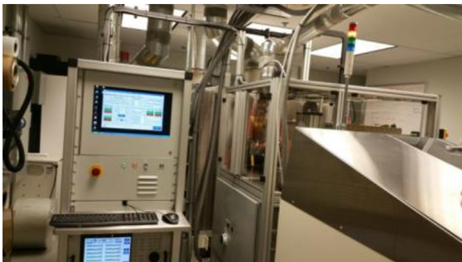
Figure 11 (a) shows the Power Module placed behind the Process Module. VFM power is transmitted and delivered by the waveguide on the top connecting the two modules.
