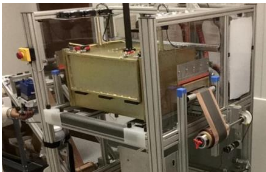
Figure 8 (b): Electrode continuously casted exits ADP process chamber completely dry.
