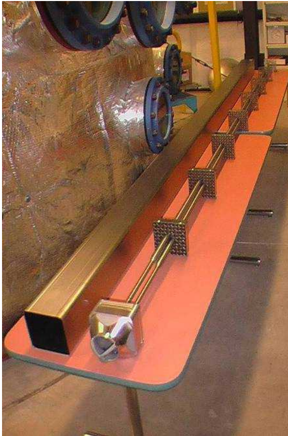
BWR channel, water tubes and spacers
