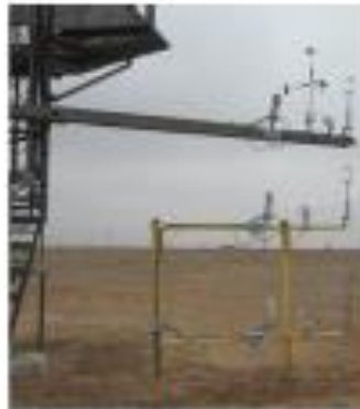
(a) Sensor Mounting at 3, 8, and 13 ft.
