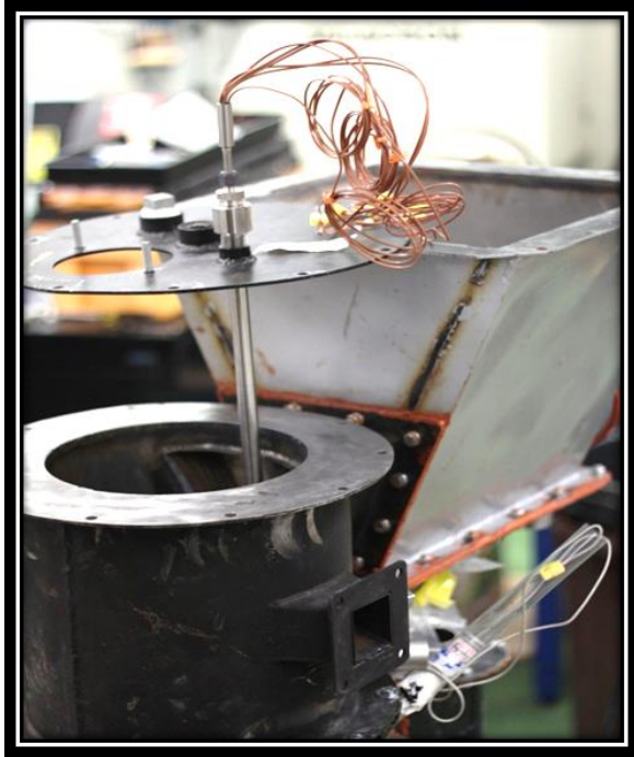
Figure (6) shows five thermal probes are installed at various locations inside the gasifier pyrolysis zone to provide thermal profile measurements – These probes are connected wirelessly to a desktop computer inside the IRTT
