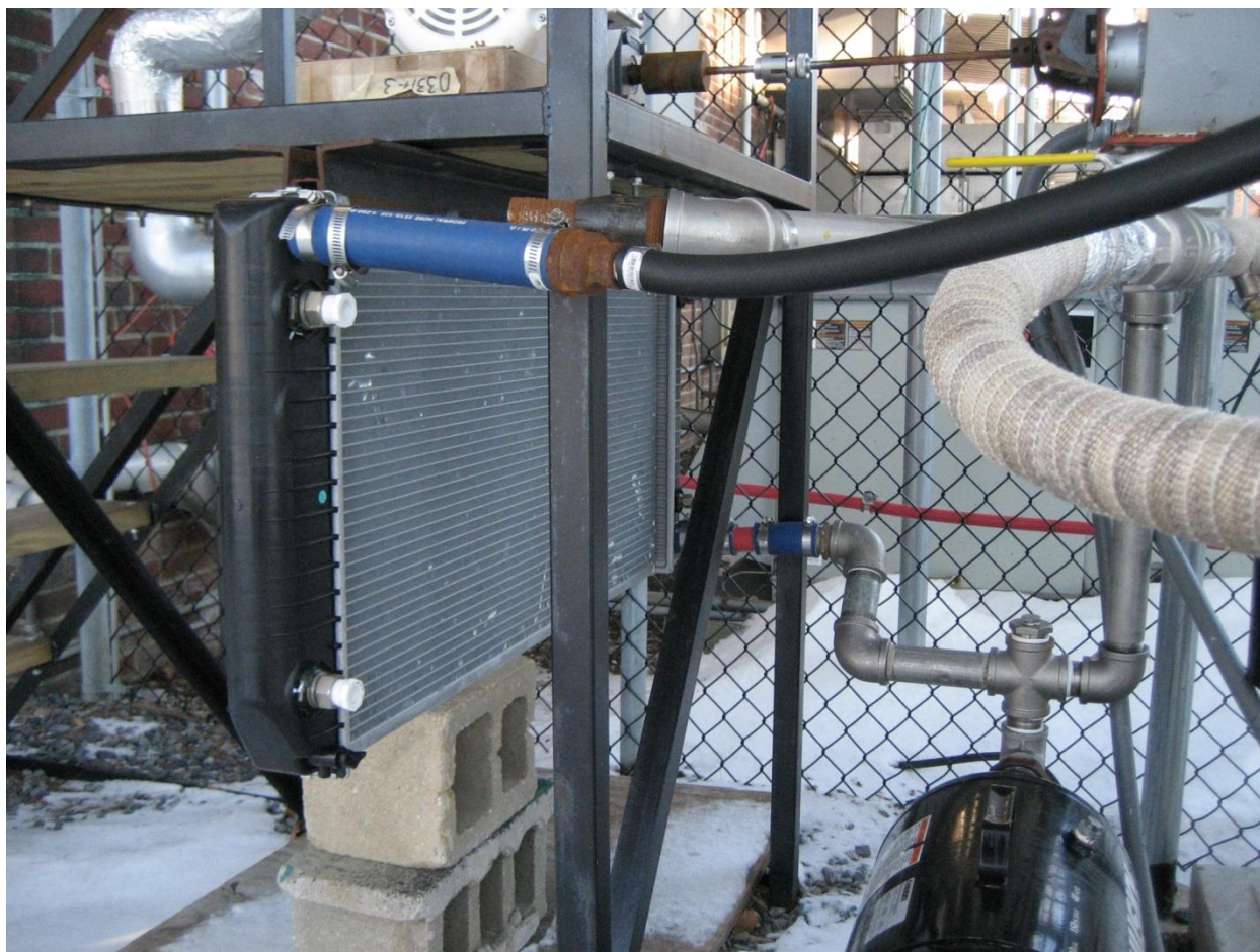
Figure (4A) Two phase separation system with cooling radiator and fan system performing in subfreezing condition
