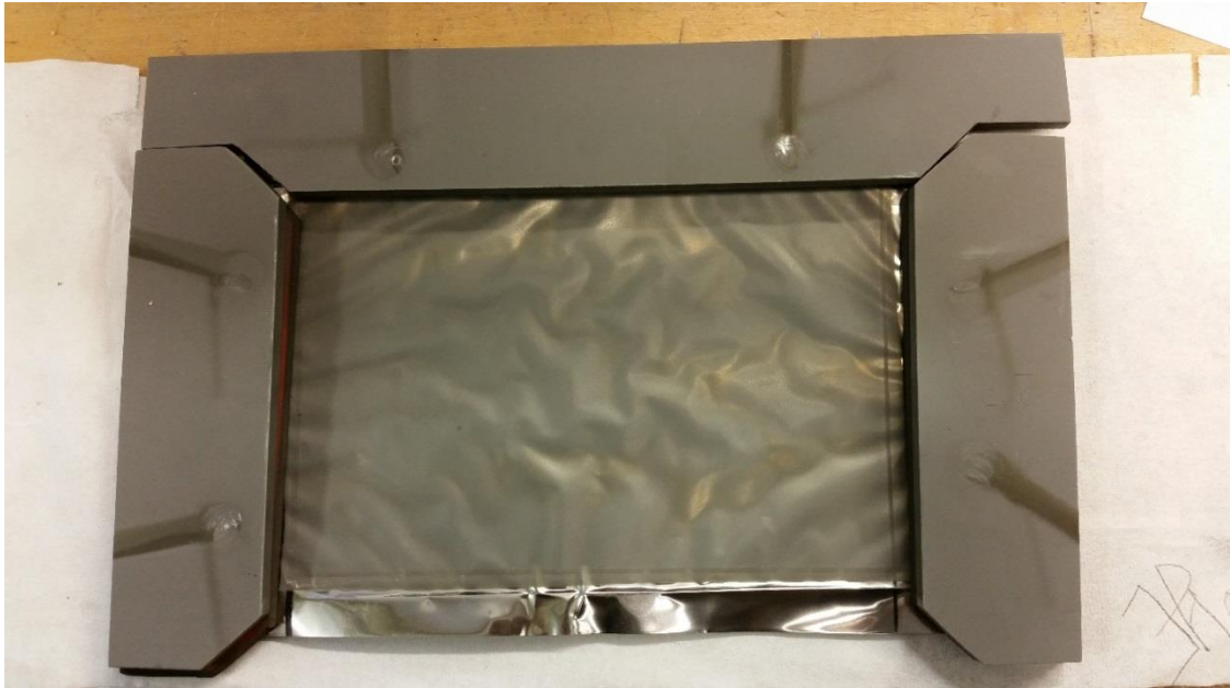
Figure (16A) Sample coated plate with excessive wrinkling- Optimization of the spray parameters is required
