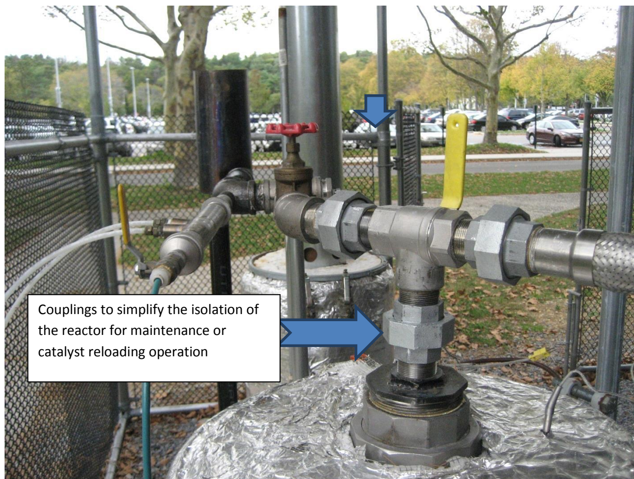
Figure (7) WGS Reactor with three added couplings to simplify maintenance process
