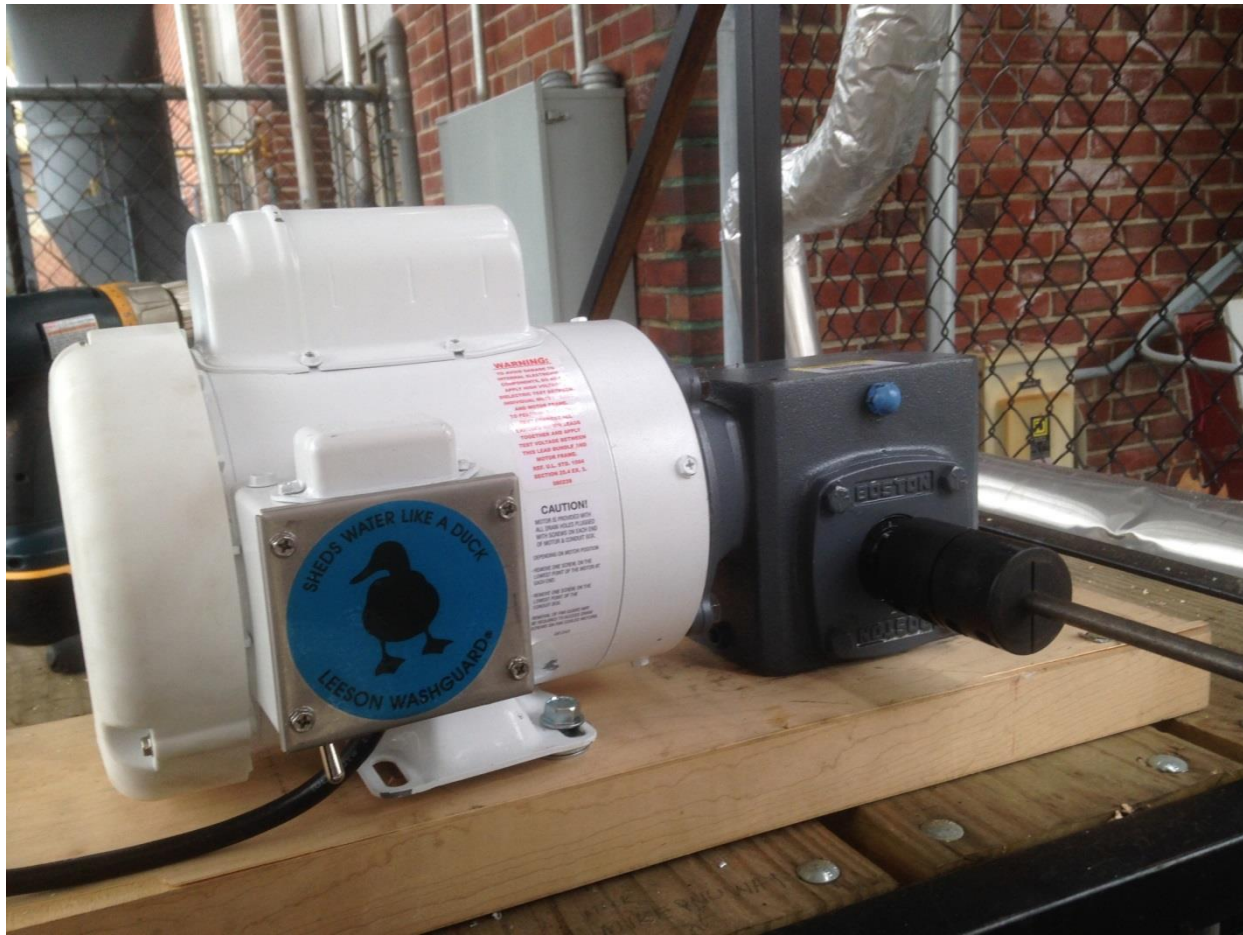
Figure (2) Close up picture of New 0.75 HP Electric Motor to power the Gasifier Auger and replace the old damaged Motor due to jammed Auger with the woodchips and exposure to electric power overload
