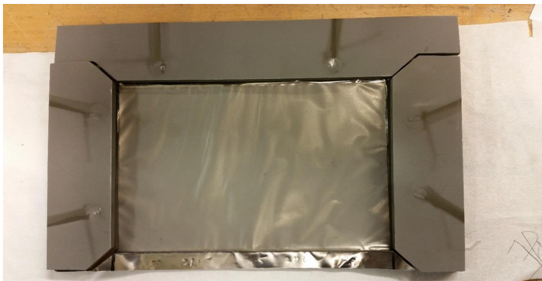
Figure (18) Sample coated plate with the least wrinkling- Optimized run #10 Table (1)
