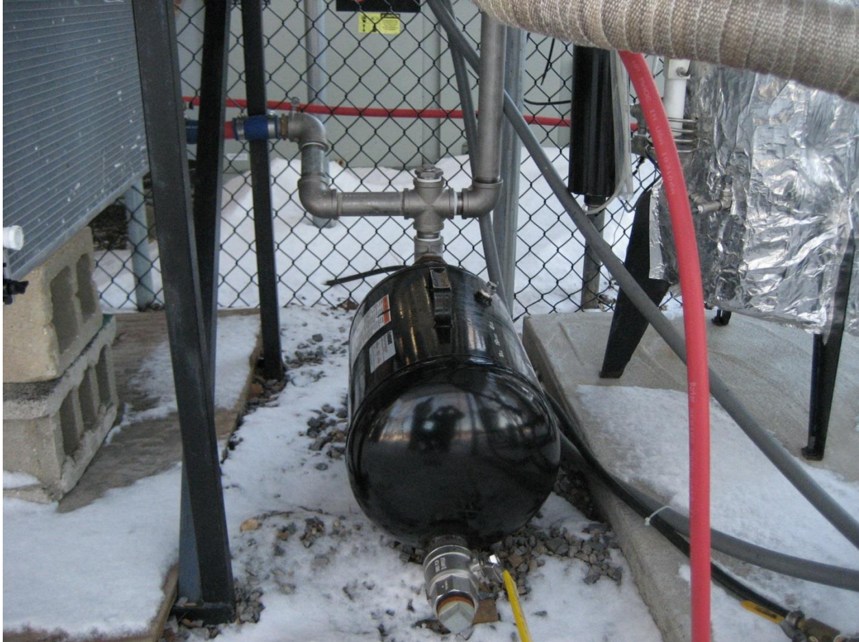
Figure (4) Two phase separation system performing in subfreezing condition
