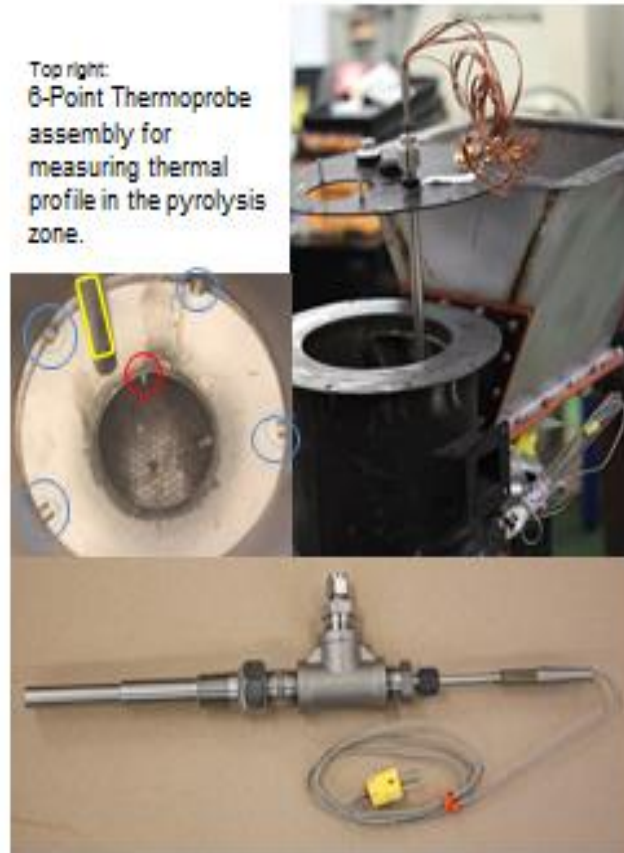
Figure (5) Sensors for Monitoring the Temperature Profile inside the Gasifier
