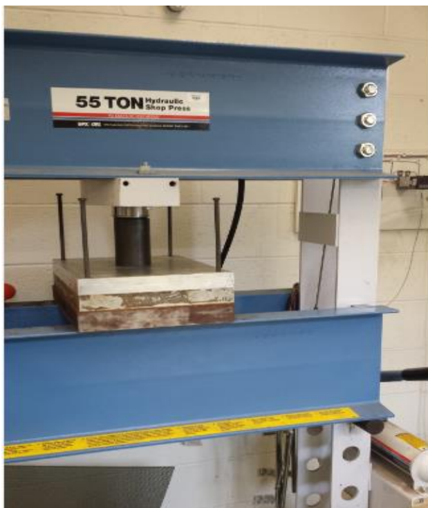
Figure (17A) 55 ton compression with heat to flatten the plate, relieve stresses and eliminate wrinkling produced by the combination of internal thermal stresses and the mismatch in the thermal expansion coefficients between the substrate and the coating materials
