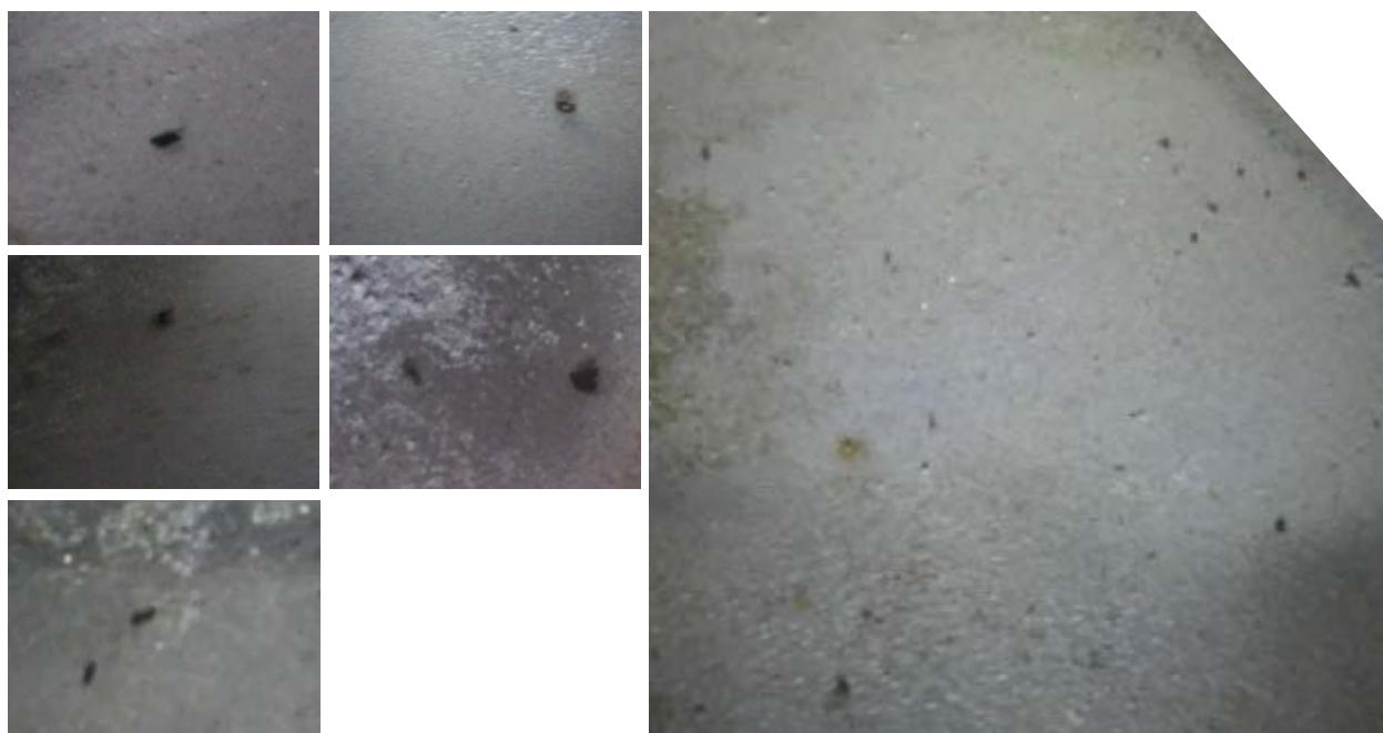
Figure 17. Boroscope camera images of insects on the floor of the HBU storage cask. The scale is not provided in the images, but comparison with structural features in the images (not shown), indicates that the insects are 2-4 mm in size. Note that each image is independent, the smaller images do not represent higher magnification views of the insects in the single larger image.
