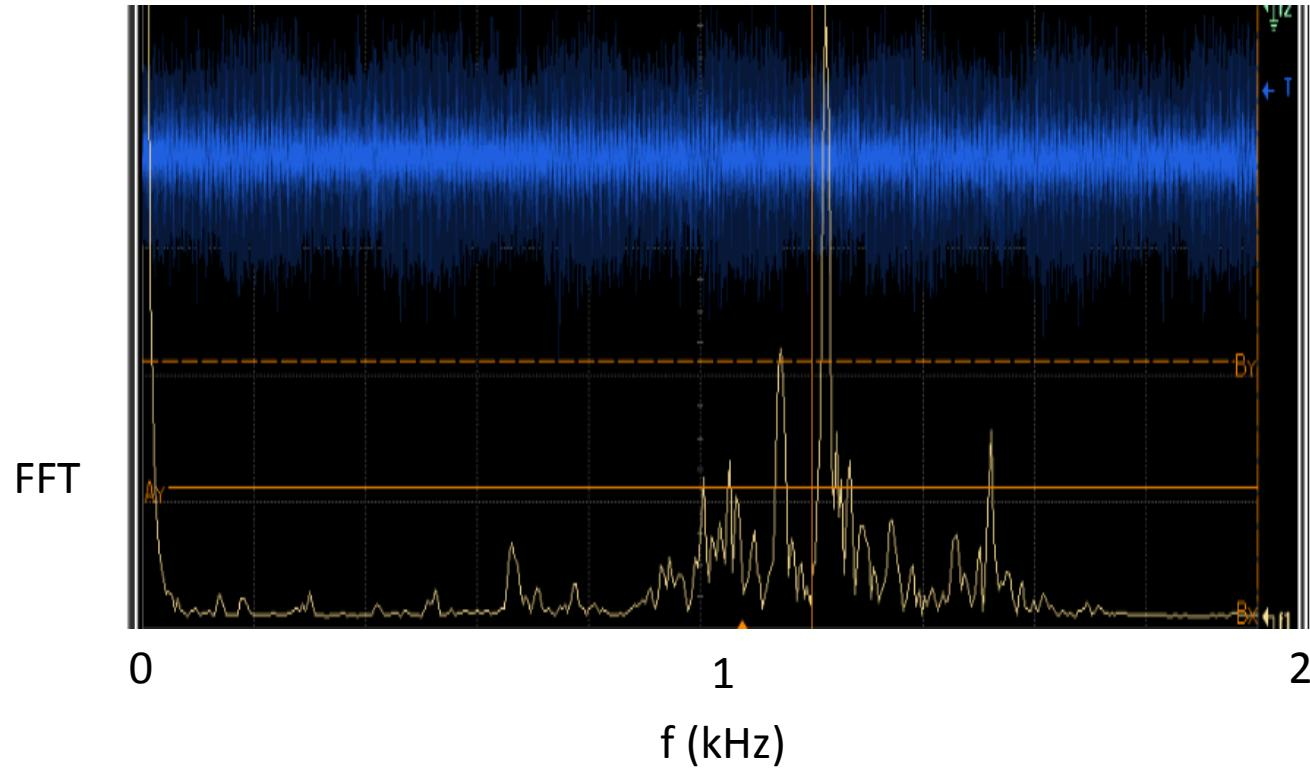
Rough estimate:  $\sim 10$   $\mu\text{m}$  of vibration,  $\sim 100$  kHz linewidth
