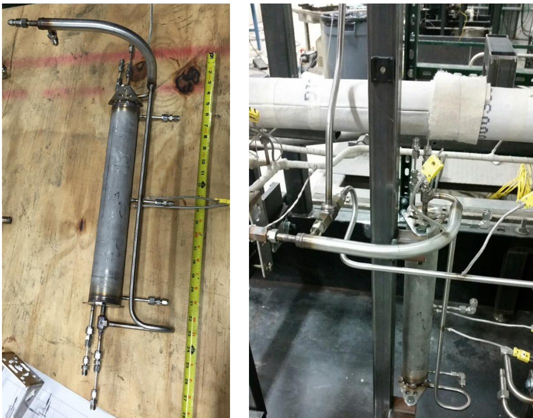
Figure 7: New cold trap with economizer
