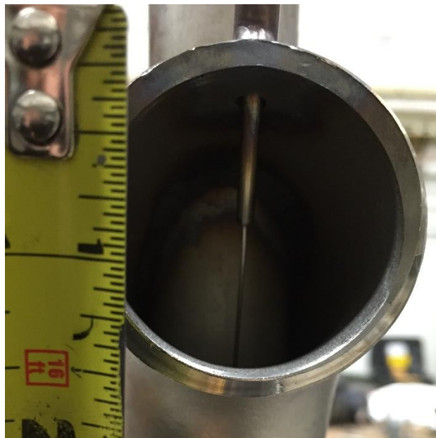
Figure 57: View of 1/8" support for capillary
