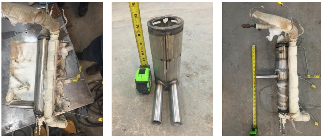
Figure 10: Cooling jacket for cold trap. Left: Original cooling jacket running full length of cold trap. Middle: Cooling jacket shortened. Right: Shortened cooling jacket installed.
