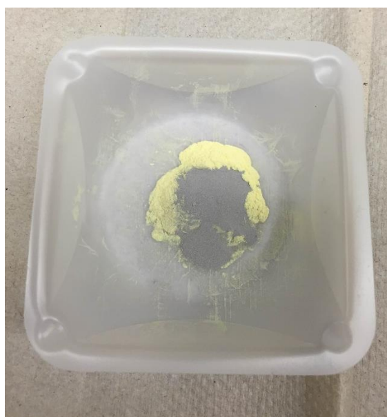
Figure 23: Indium/Indium Oxide Mixture Prior to Filling Sensor Electrode
