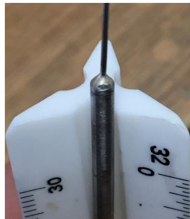
Figure 55: Silver solder joint, 1/8" tube to 1/32" capillary
