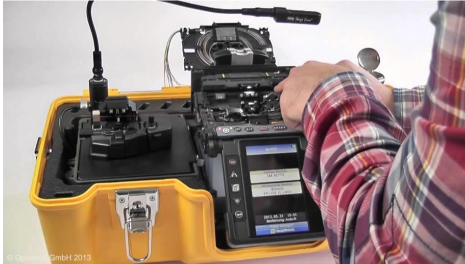
Figure 51: Fujikura 70s Fusion Splicer with AFL CT-30 Precision Fiber Optic Cleaver
