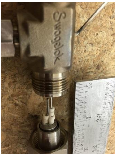
Figure 22: Molybdenum Wire and Internal Thermocouple with Alumina Spacers
