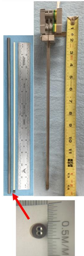
Figure 33: UW built continuous electric level sensor
