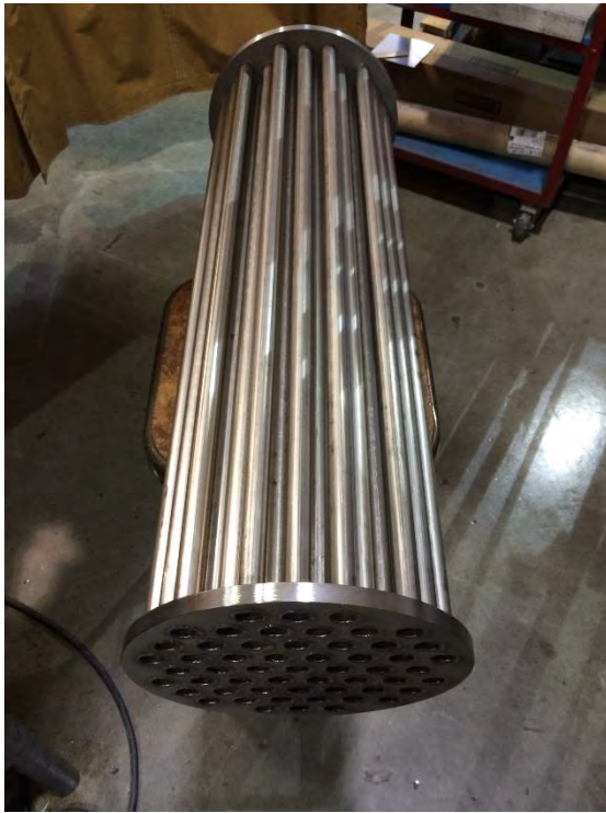
Figure 11-8 Design of ESF Steam Generator
