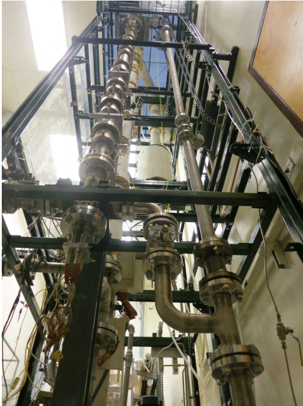
Figure 4-10 Natural Circulation Instability Facility before Insulation
