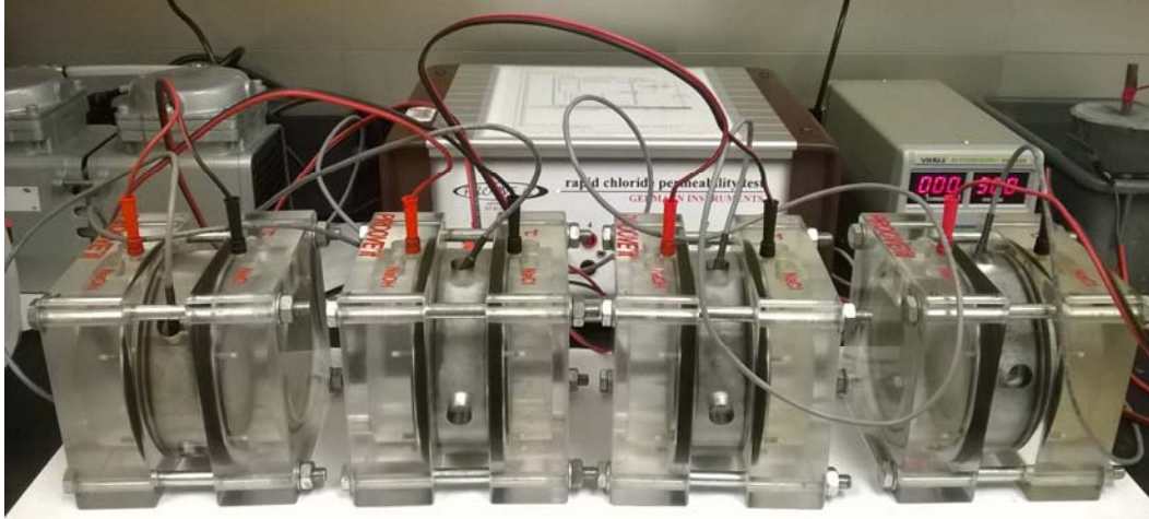
Figure 7.4. Rapid chloride permeability test measurement in progress
