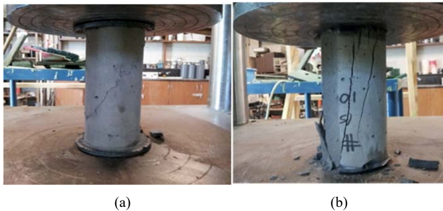
Figure 2.17: Compressive failure mode of (a) SHC and (b) normal concrete
