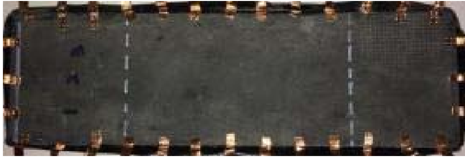
Figure 4.32. Specimen before damage with 32 electrodes.
