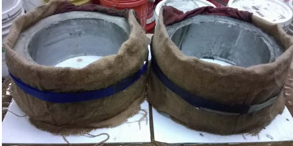
Figure 7.11: Specimen moisture-curing with a burlap
