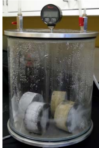
Figure 7.2. Conditioning of specimens with a vacuum desiccator
