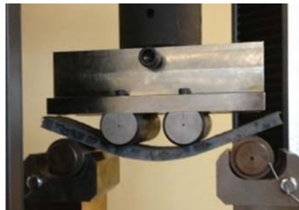
Figure 2.19: A highly deformed SHC specimen under four point bending; no steel reinforcement was used.
