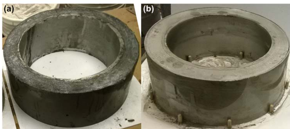
Figure 7.10: Casted restrained shrinkage specimens of (a) MSC and (b) control concrete.
