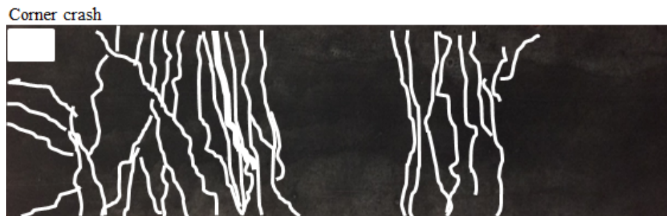
Figure 4.29: Damage pattern illustration of 5% MSC material specimen No.(3).
