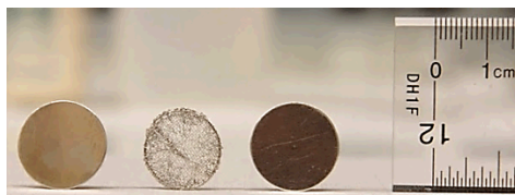
Figure 1. Three platinum electrodes used as anodes in electrodeposition. From left: solid disc electrode with thin wire stem, mesh electrode with thin wire stem, and solid disc electrode with thick wire stem.
