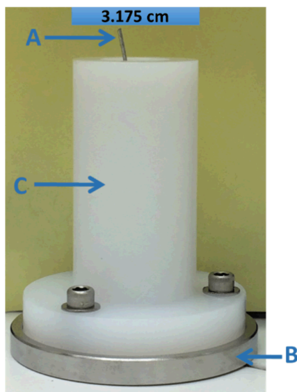
Figure 3. Teflon chimney molecular deposition cell. A: Stem of platinum electrode inserted into cell. B: Stainless steel cell base with inset (not visible) for aluminum disc. C: Teflon chimney.
