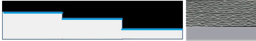
Fig. 1. Specimens are constructed of carbon fiber reinforced plastic (CFRP) [4 ply [0/90]_2 ] s , 8 ply [0/90]_4 ] s and 12 ply [0/90]_6 ] s preimpregnated 8 harness-satin weave with UF3352 TCR™ Resin
