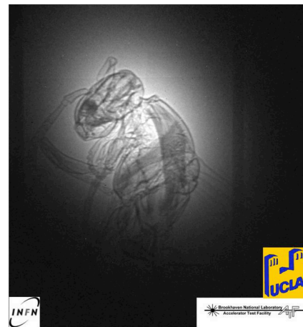
Figure 10. Radiograph of wasp made by narrow-band ICS X-rays, showing phase contrast effect at boundaries.
