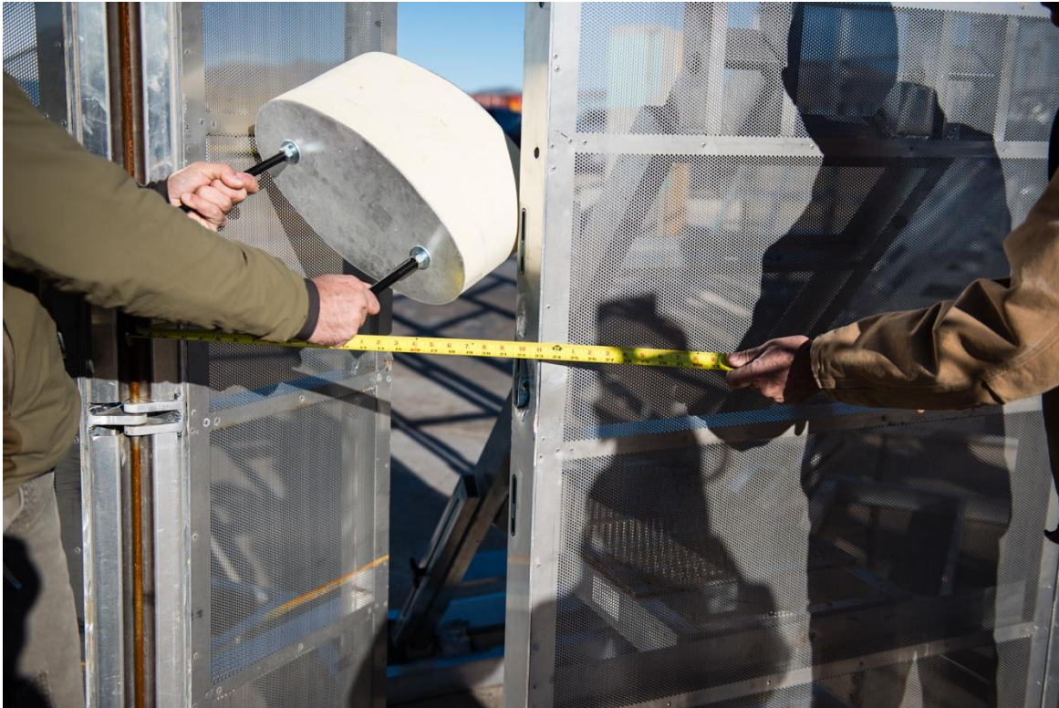
Figure 68 Ellipse used to determine test completion during test 19
