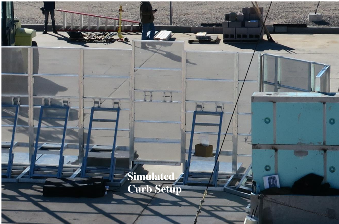
Figure 37 Simulated curb/median setup during barrier effectiveness testing
