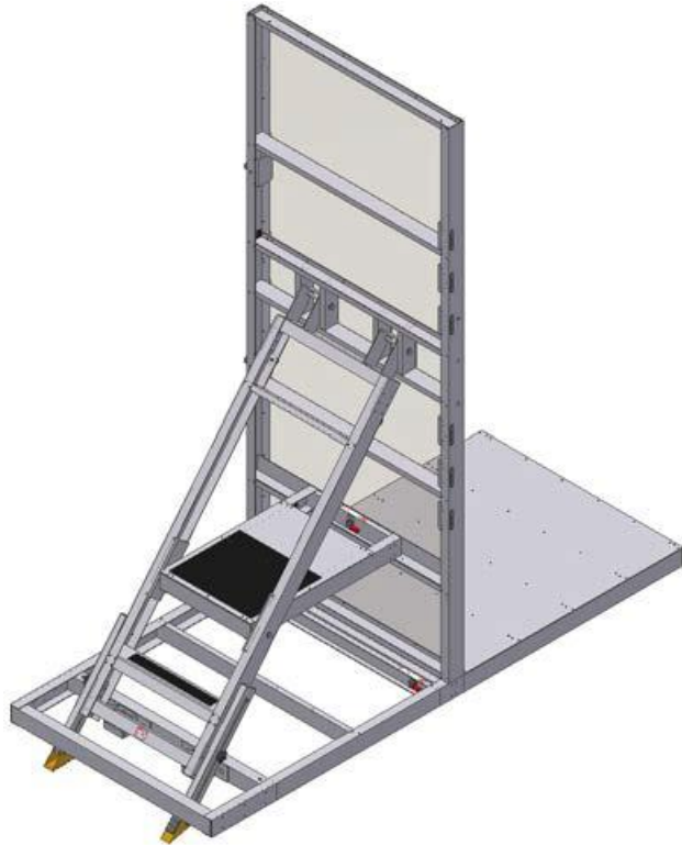
Figure 14 Rendering of the full base and upright assembly in an assembled position (straight section) [ref 9]
