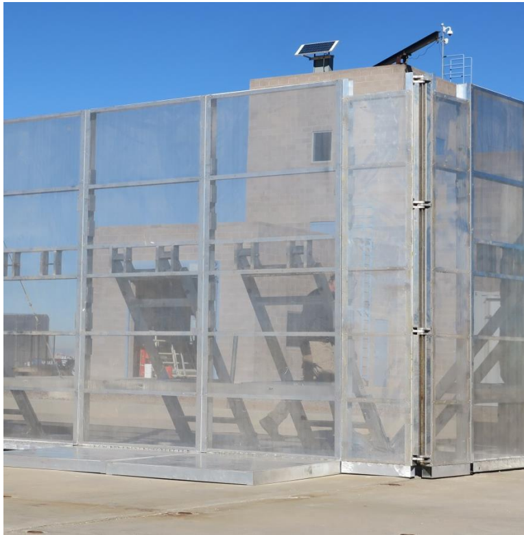
Figure 34 Compact 90-degree turn during barrier effectiveness testing
