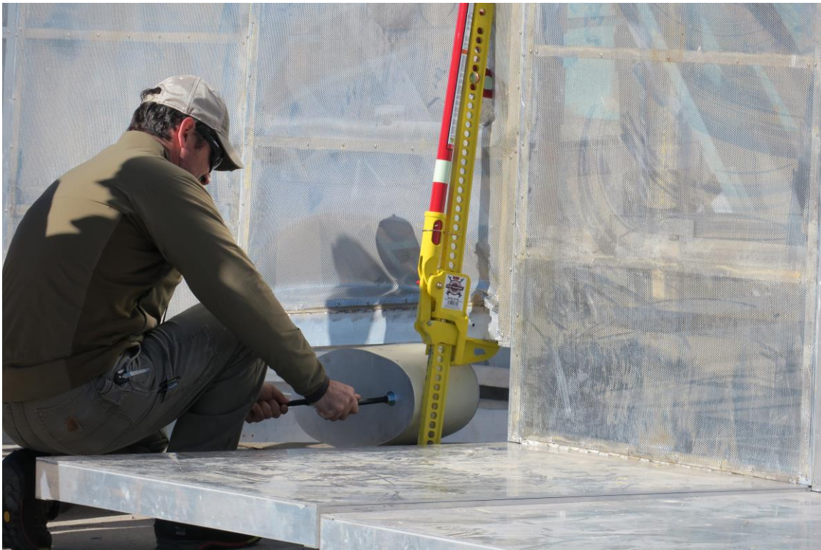
Figure 67 Breach test using the hydraulic jack-lift during test 9
