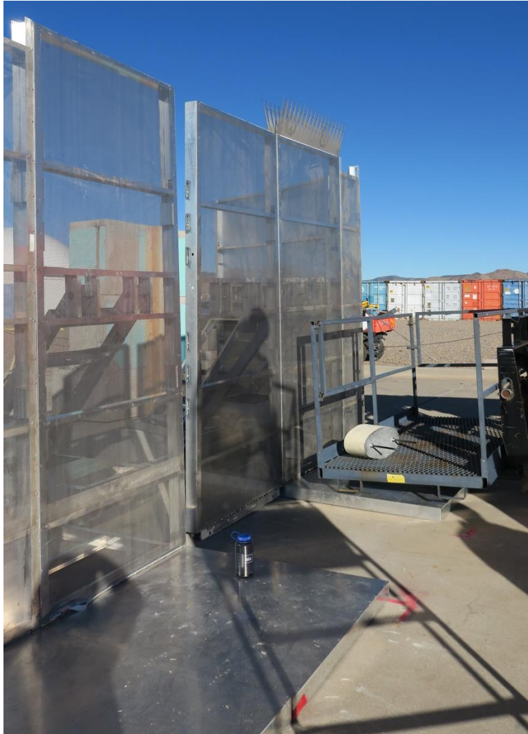
Figure 13 Spikes installed atop upright during barrier effectiveness testing
