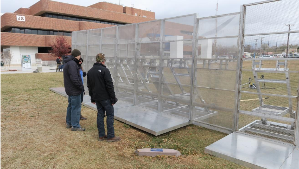
Figure 39 TAP barrier deployed over a drainage slope during deployment efficiency testing
