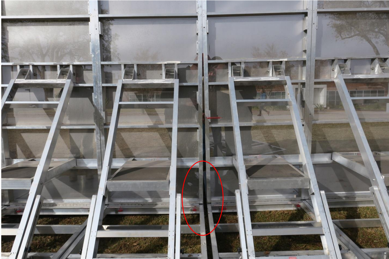
Figure 48 Test 4 configuration showing the component that was not properly latched due to issues with the quick lock not catching
