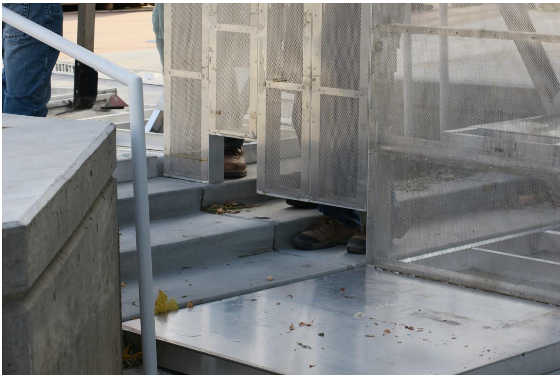
Figure 36 Adapter component assembled over stairs during deployment efficiency testing (cont'd.)
