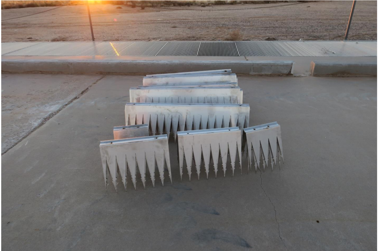
Figure 12 Spikes that were available during barrier effectiveness testing (not assembled on upright)
