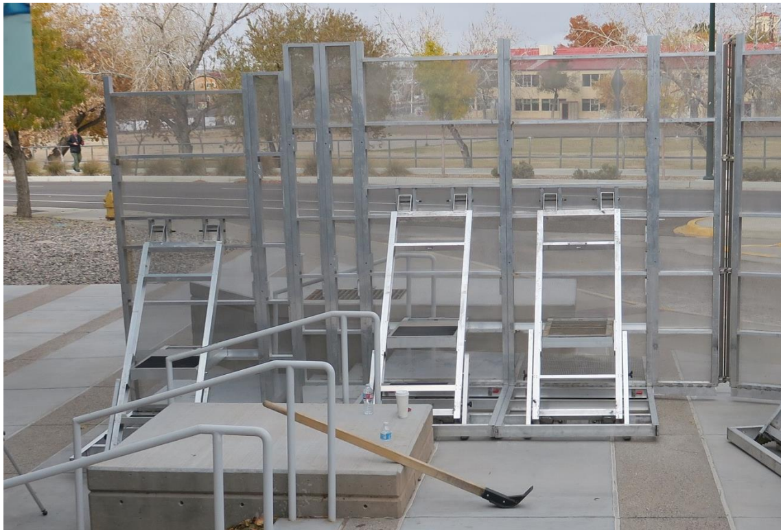
Figure 35 Adapter component assembled over stairs during deployment efficiency testing
