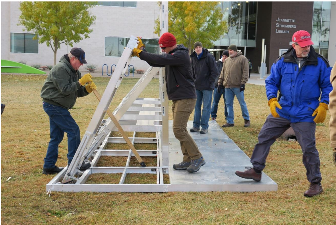
Figure 17 Crowbar leveling tool being used during deployment efficiency testing
