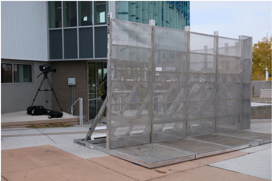
Figure 38 TAP barrier deployed up a slope during deployment efficiency testing
