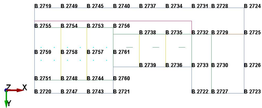
Figure 2-10: Plan layout of isolators for the GDNF
