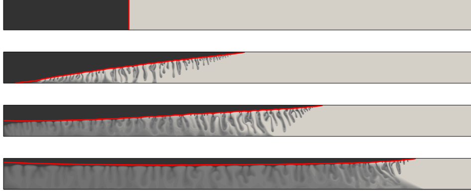
Figure 14. Sequence of snapshots from a high-resolution simulation of convective dissolution from a buoyant current in a sloping aquifer for Ra = 5000 , R = 1 , and \theta = 2.5^\circ (not shown) at dimensionless times 0, 3, 9, and 27. The domain extends to x = 20 , but only 0 \leq x \leq 15 is shown here. The red line marks the contour of neutrally buoyant concentration c = c_n , which separates the buoyant current from the sinking fluid.
