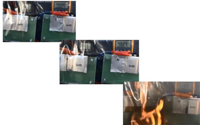
Figure 43 Photos of cells containing hydrocarbon (left) and fluorocarbon (right) electrolyte at 10, 1400, and 1500 seconds overcharging.
