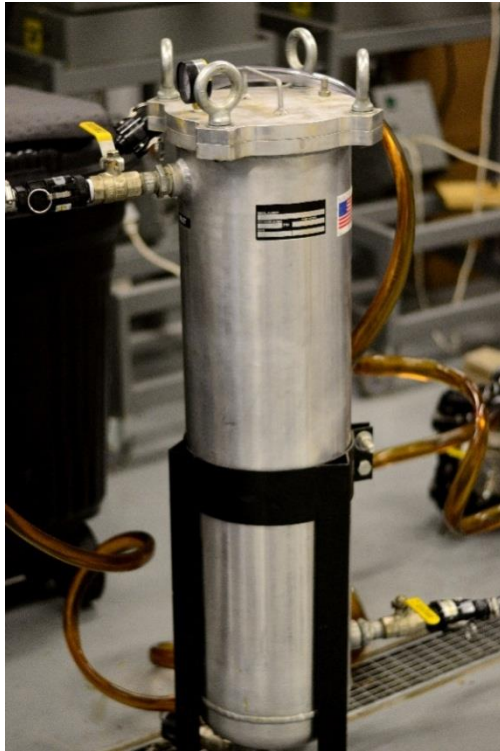
Figure 8. Primary filtration unit. (a) Left photo: Bio-Energy Center's primary filtration setup with a 50µm polyester filter bag inside. (b) Top photo: Schematic illustration on how solids are removed from an oil during filtration.
