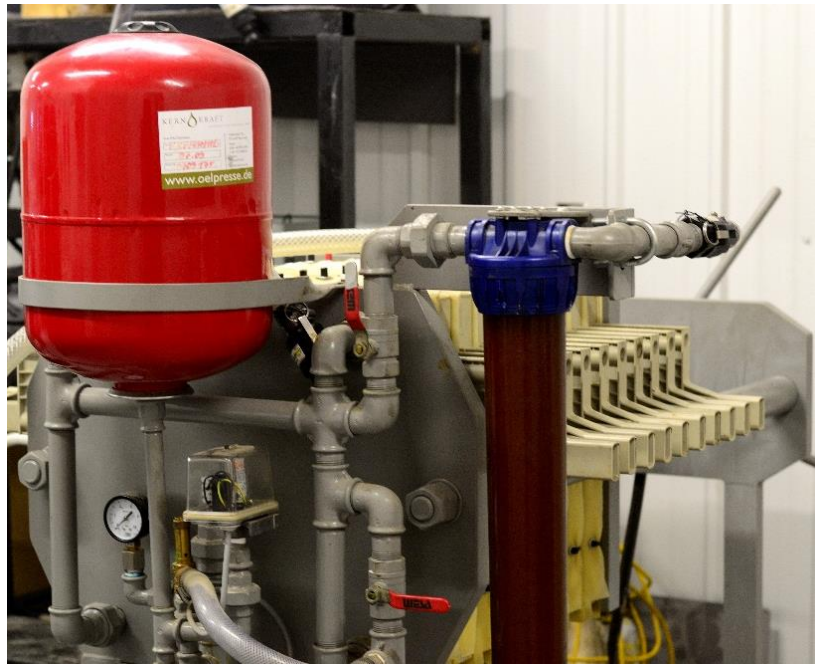
Figure 9. Filter press unit. (a) Left photo: Schematic illustration on how solids are removed from an oil in a filter press. (b) Right photo: Bio-Energy Center's filter press unit.
