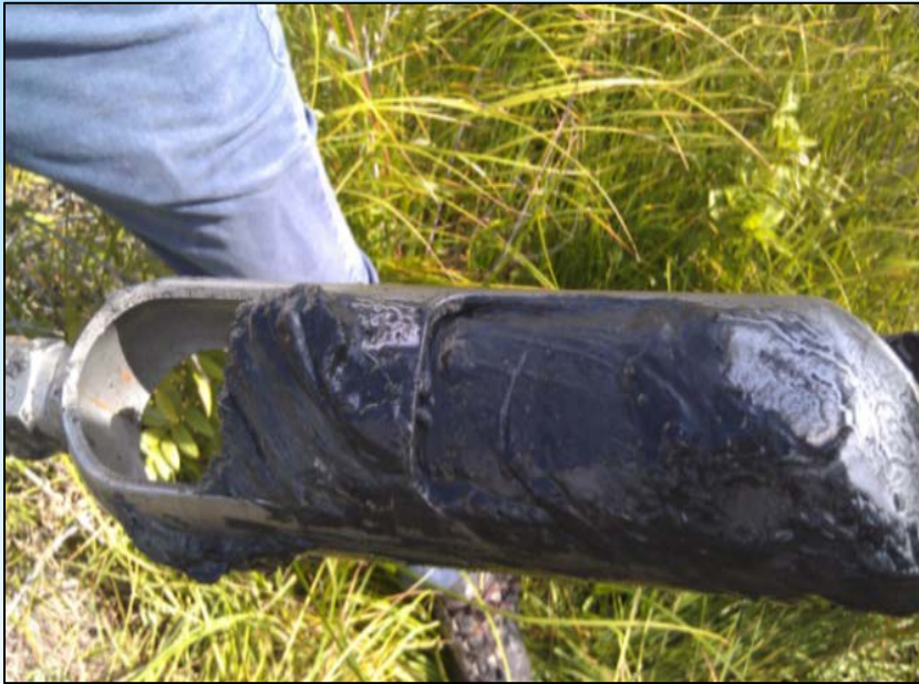
Hand-augered core in oxbow sediments
