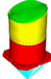
Figure 3 – Predicted elastic mode shapes of test article affixed to seismic mass.
