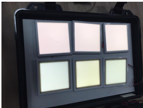
Figure 6. A small demo showing both LGD (top) and OLEDWorks (bottom) panels driven in the same string
