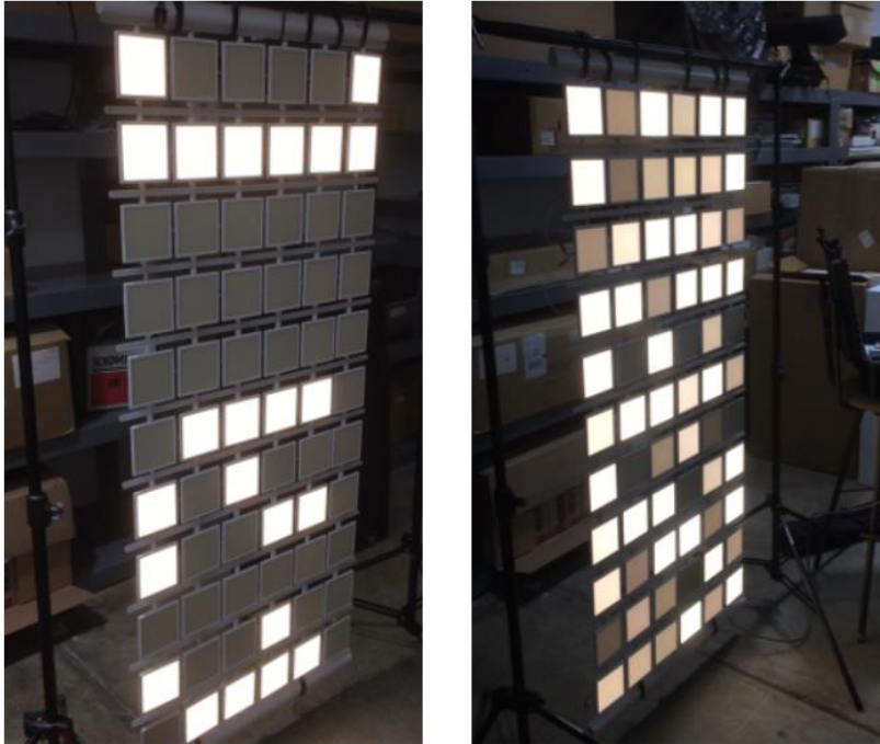
Figure 7. Full size Canvis demo fixture with individual panel addressing. Two control modes are shown: scrolling text (left) and rain drop (right)
