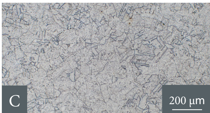
Micrographs of 316L stainless steel (SS): a) annealed wrought plate; b) additive manufactured (AM) (as-built); c) AM following recrystallization heat-treatment at 1060 °C for one hour. Research showed that the spall strength—the ability to resist damage—of additively manufactured 316L SS was similar to that of the annealed wrought or AM-316L SS following recrystallization for high shock pressures, but all three were significantly different for lower loading pressures.
