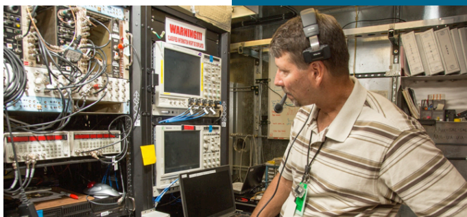
A National Security Technology (NSTec) researcher tests one of several multiplexed photonic Doppler velocimetry systems underground in Nevada. The close collaboration of Los Alamos and NSTec ensures acquisition of high-quality data under challenging experimental conditions.
