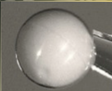
Above: foam target for an OMEGA experiment. The capsule diameter is approximately 1.7 mm.
