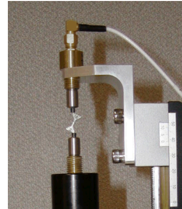
dogbone in the 2-point test fixture
