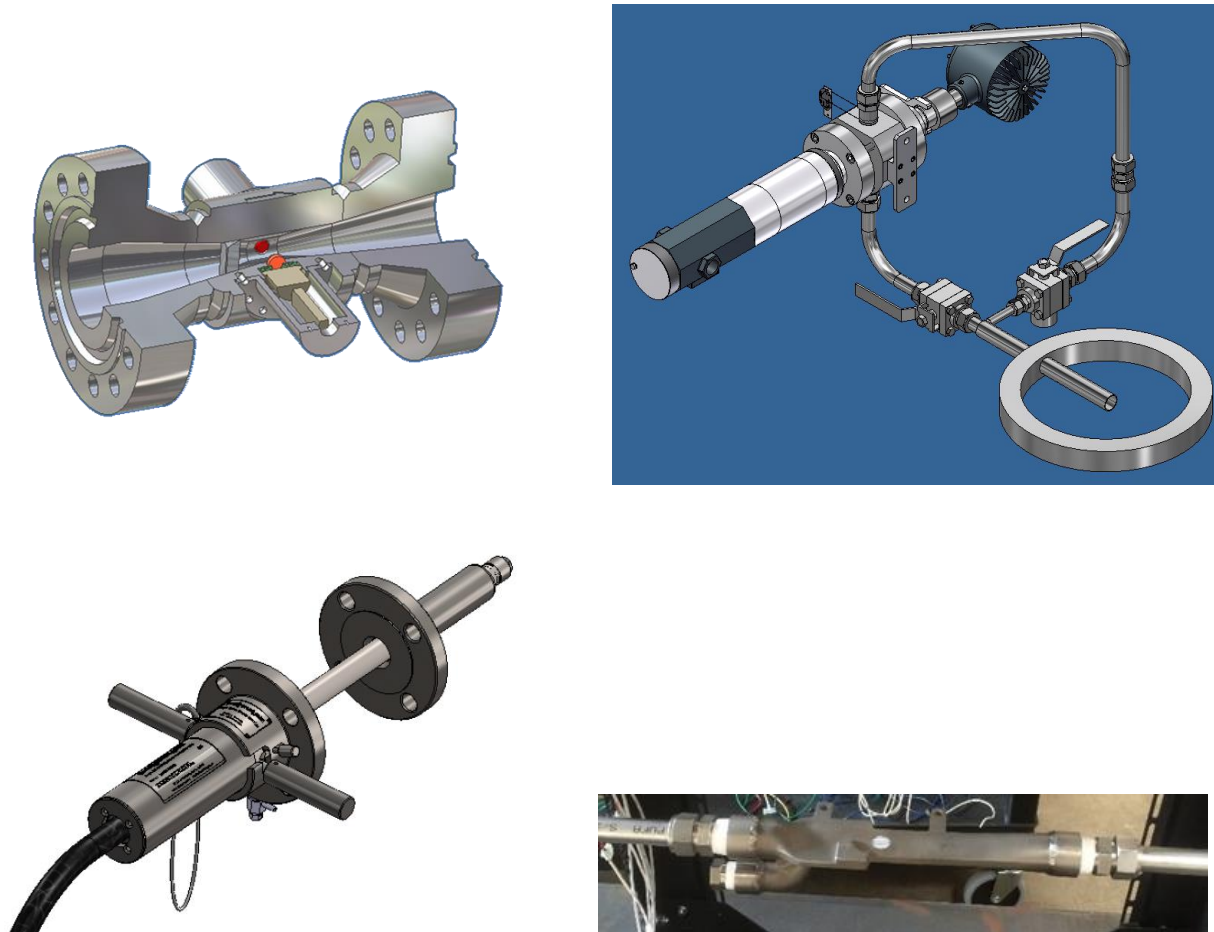
Figure 72: Digitrol sensor (Top Left); JM Canty Produced Water Quality Monitor prototype (Top Right); Proanalysis OIWM Probe prototype (Bottom Left); and Measurement Section with Sapphire Windows, Connection to Sample Piping, and Connection to Cleaning Water Piping portion of Clearview Subsea Confocal Laser Fluorescence Microscopy prototype (Bottom Right).
