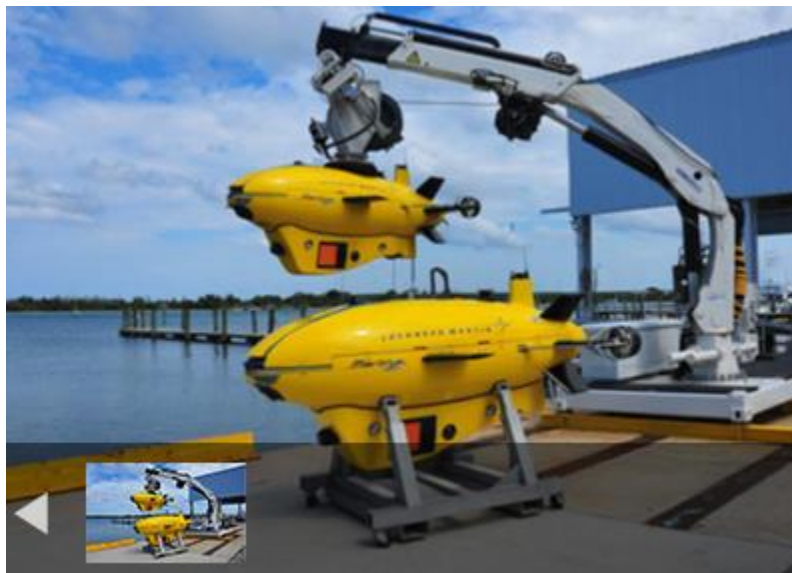
Figure 68: Photo of Lockheed Martin’s commercialized Marlin AUV’s (courtesy of Lockheed Martin).
