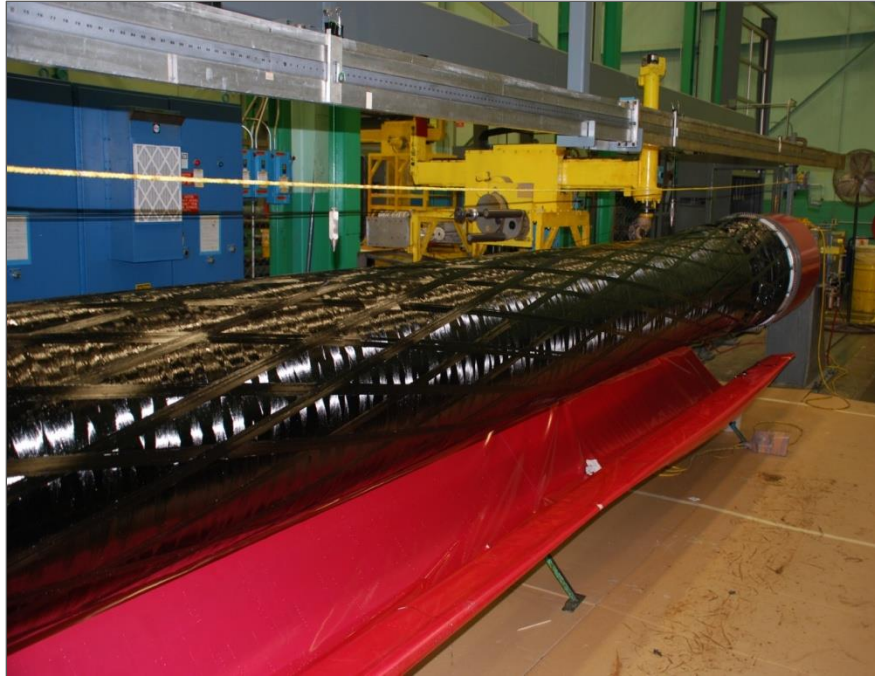
Figure 12: Winding the composite riser prototype
