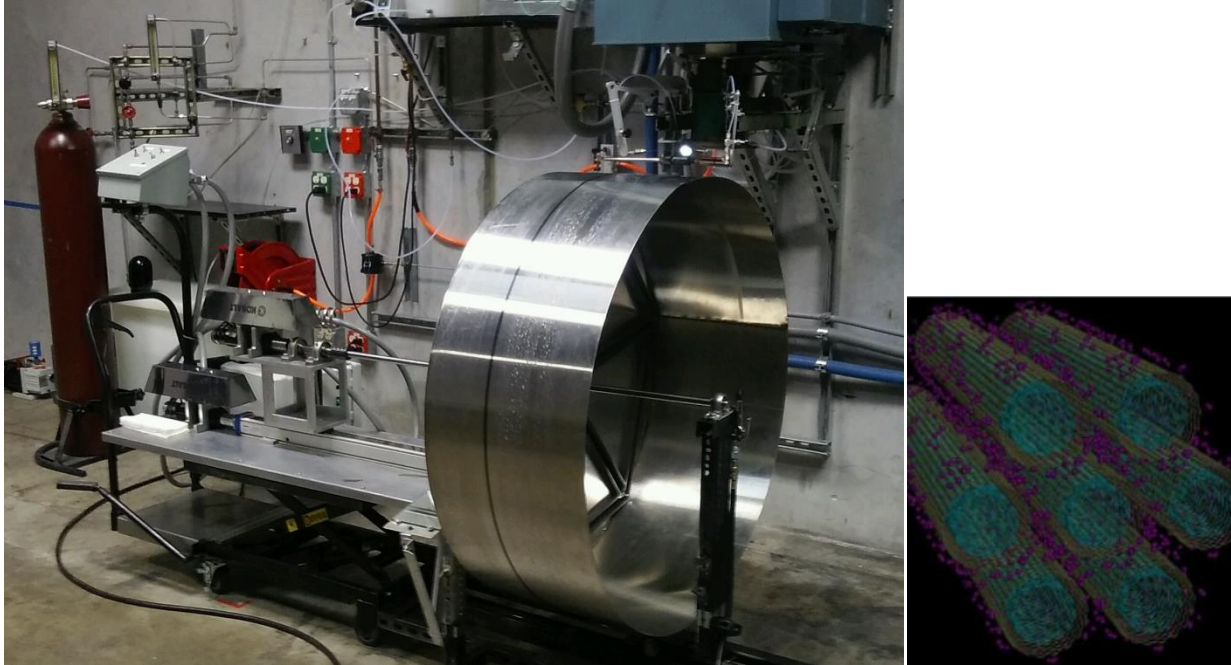
Figure 58: Photo of newly manufactured carbon nanotube wire on a drum spool.
