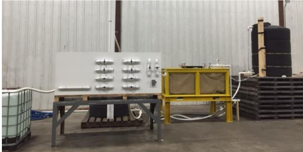
Figure 73: Subsea compensated chemical reservoir scale model prototype test apparatus (yellow) with fluid tanks and controls.
