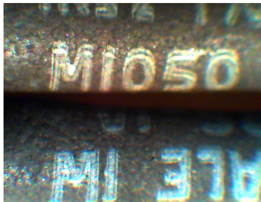
R2: Cheap "China" 2.2k\Omega // 2.2k\Omega (parallel). Again, notice the discoloration.
