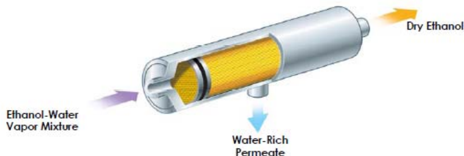
Figure 20: Vaperma Siftek Distillation Technology Concept
