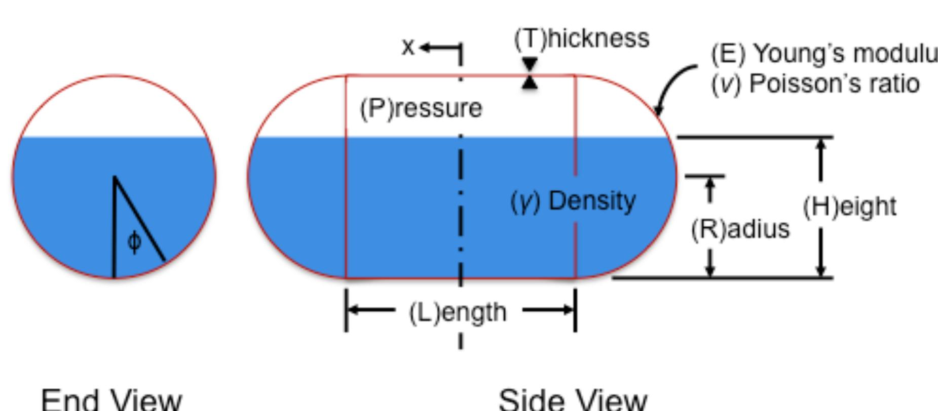
Specifically, what is the probability that the maximum von Mises stress exceeds the yield stress under nominal operating conditions?
