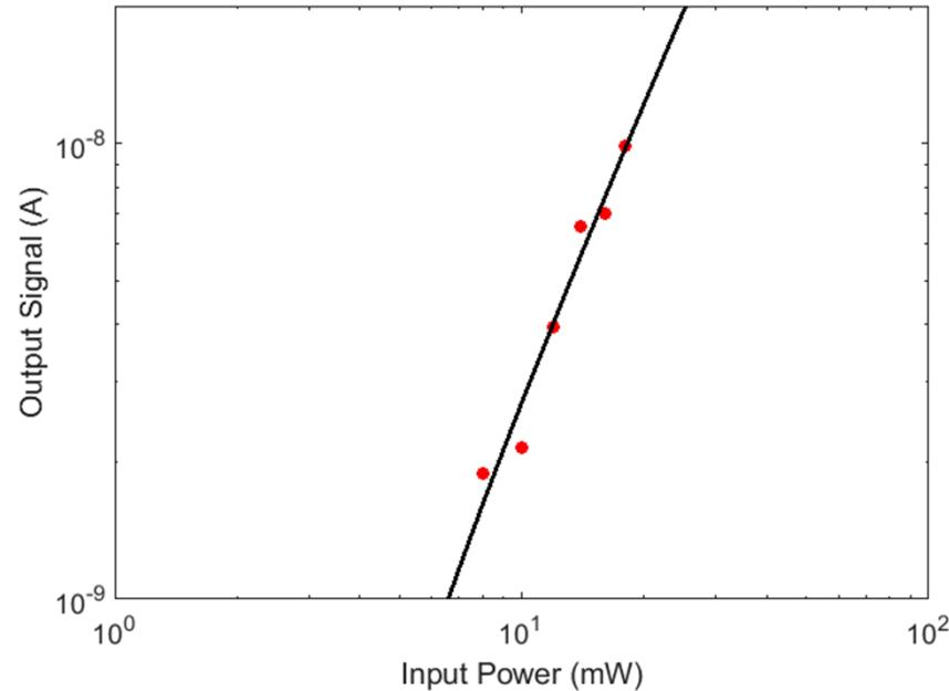
Pump power vs. generated 2<sup>nd</sup> harmonic generated power
