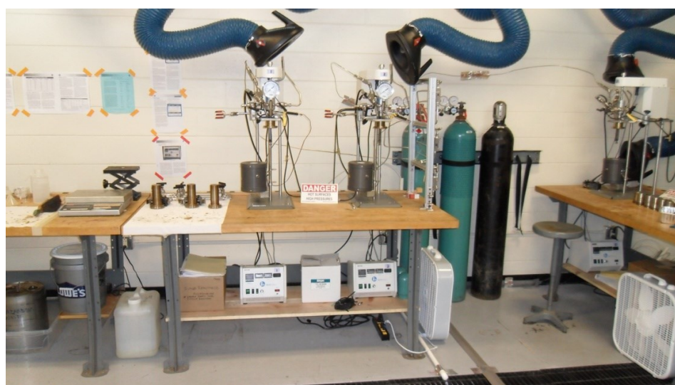
Figure 4: Catalytic test bed for algae liquefaction and algal oil upgrading studies (A-low temperature, pressure system [300°C, 3000 psig, max]; B-high pressure, temperature [500°C, 5000 psig, max] system).
