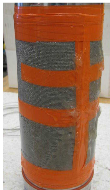
Fig. 2. Specimen with end caps and wrapped in the steel frit material. The orange electrical tape is used to close the frit around the specimen and to connect the specimen, end cap and
