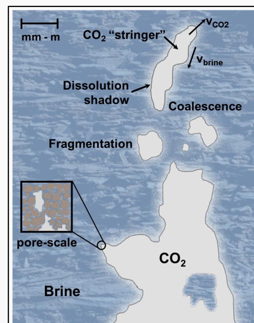
Figure: Conceptual model and mechanistic processes in buoyancy-driven ganglion dynamics (note  $v_{CO_2}$ ,  $v_{brine}$  of "stringer") which collectively correspond to capillary channelling.
