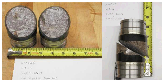
Fig. 4. Saw cut surface on sample NG-4 240.5 (strongly welded tuff).
