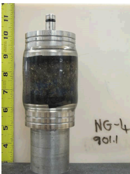
Fig. 5. Sample NG-4 901.1 (rhyolitic lava) shown with vented endcaps.
