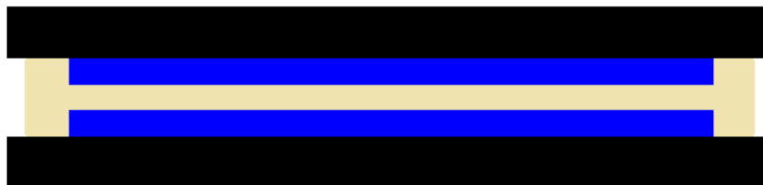
Figure 8.8. Intrapore density is calculated by taking volumetric storage capacity and dividing by the sample porosity. Intrapore density \rho_{ip} of the adsorbent includes both the adsorbed film (blue) on the sorbent surface (black) plus non-adsorbed gas (tan) in the pore space.
