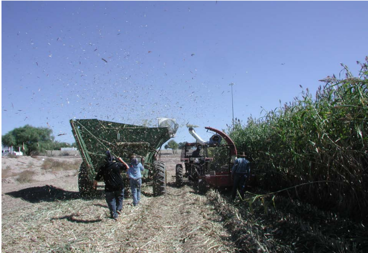
Figure B1. Modified forage chopper harvesting sweet sorghum.
