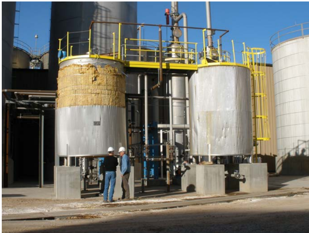
Figure D1. 10,000 cone bottom fermenters for sweet sorghum juice at Pinal Energy, LLC.
