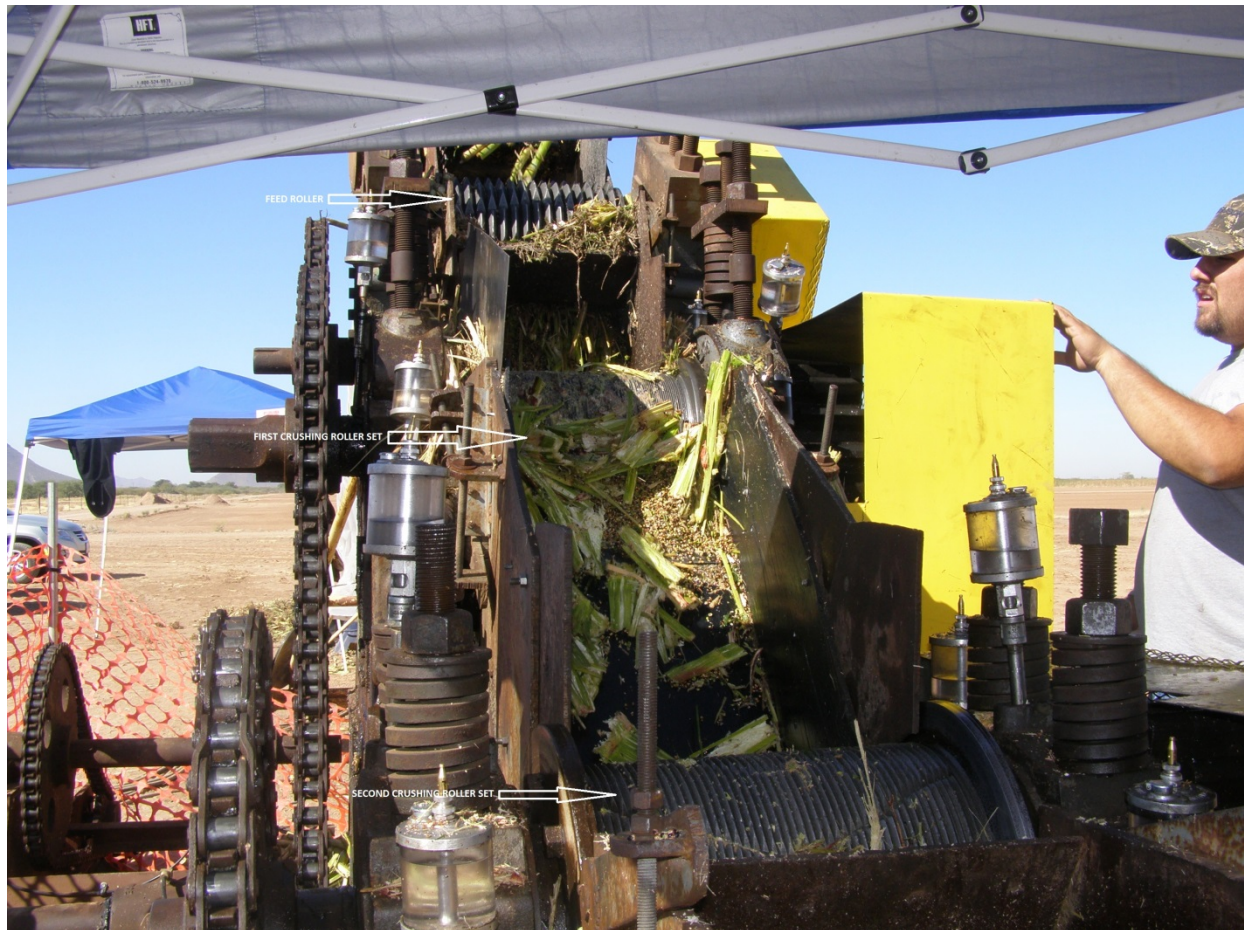
Figure C3. Leased mill in operation showing three sets of rollers.
