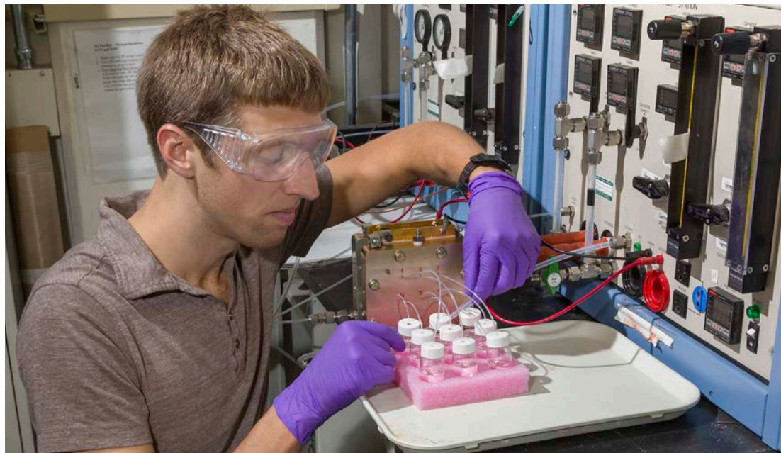
Jacob Spendelow preps a reference electrode setup connected to a fuel cell enclosed in hardware. The setup measures electric potential at nine different points on the cathode and can gauge impurities as well as potential degradation affecting its performance.
