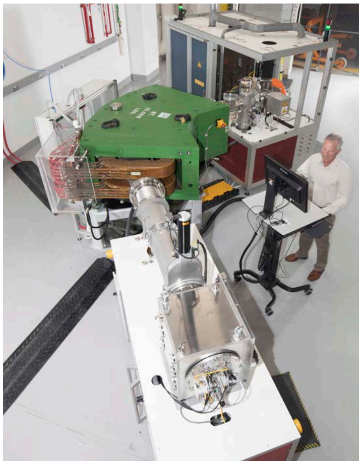
Los Alamos researchers in collaboration with external colleagues have successfully developed and tested a high-throughput electromagnetic isotope separator (EMIS) capable of producing gram-scale quantities of high purity isotopes in a single day.
