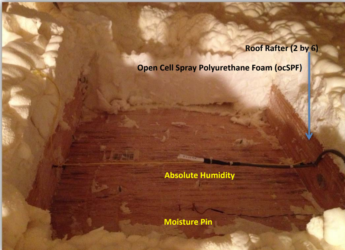
Fig. 5. The sheathing on the north facing roof deck. Open cell spray polyurethane foam insulation removed to inspect sheathing and add instruments after 2 years of climatic exposure.
