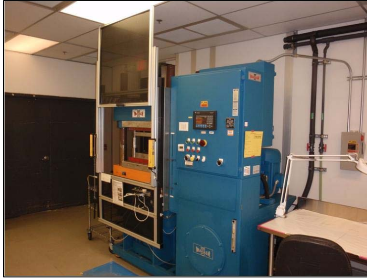
Figure 11 Press used to bond the sub-layers through applied heat and load.
