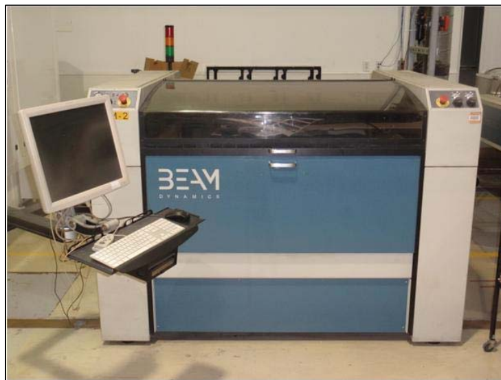
Figure 12 Laser station at Ceramatec utilized to accomplish microchannel featuring of each distinct sub-layer within Design 1.2 heat exchange plates.
