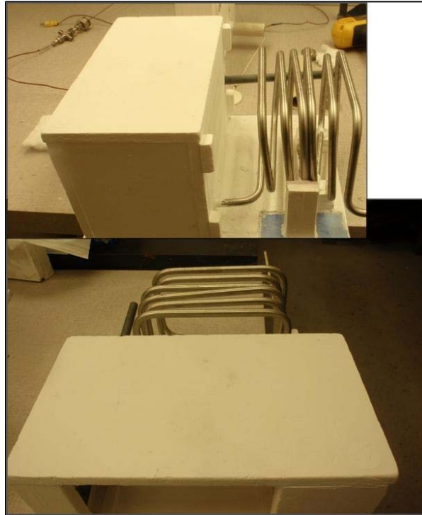
Figure 27 Coiled (10.5 linear feet) 304 stainless steel pre-heater replacing the alumina pre-heater unit.
