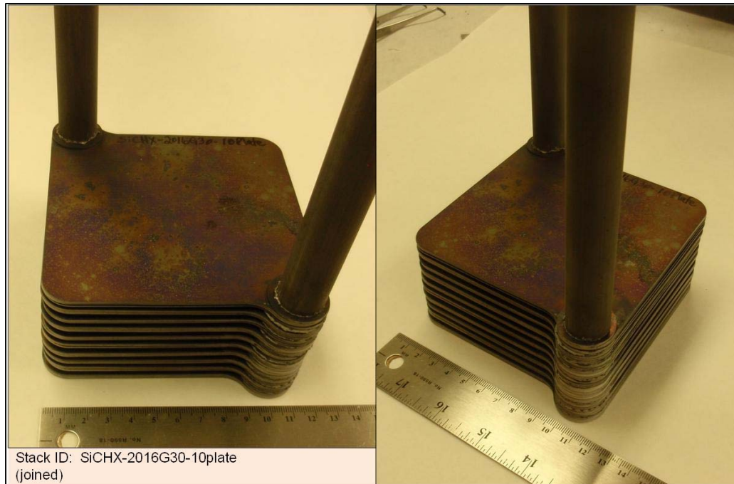
Figure 24 Fully joined 10-plate SiC HX stack (with inlet and outlet flow tubes).
