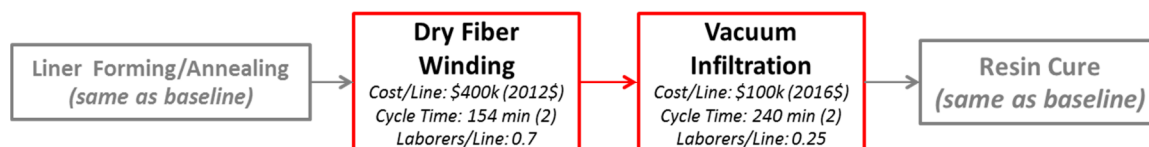
Figure 14: Manufacturing process flow for vacuum infusion.
