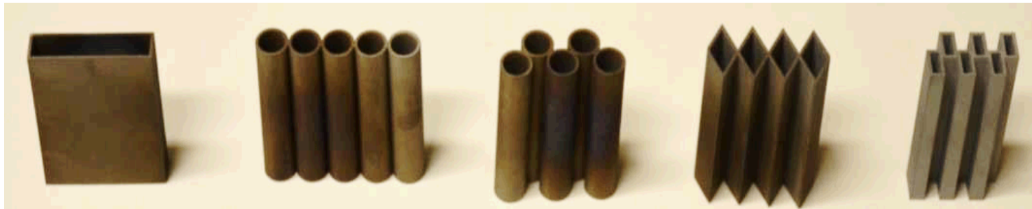
Prototype fractal-like geometries (FLGs) fabricated with additive manufacturing using Inconel 718
